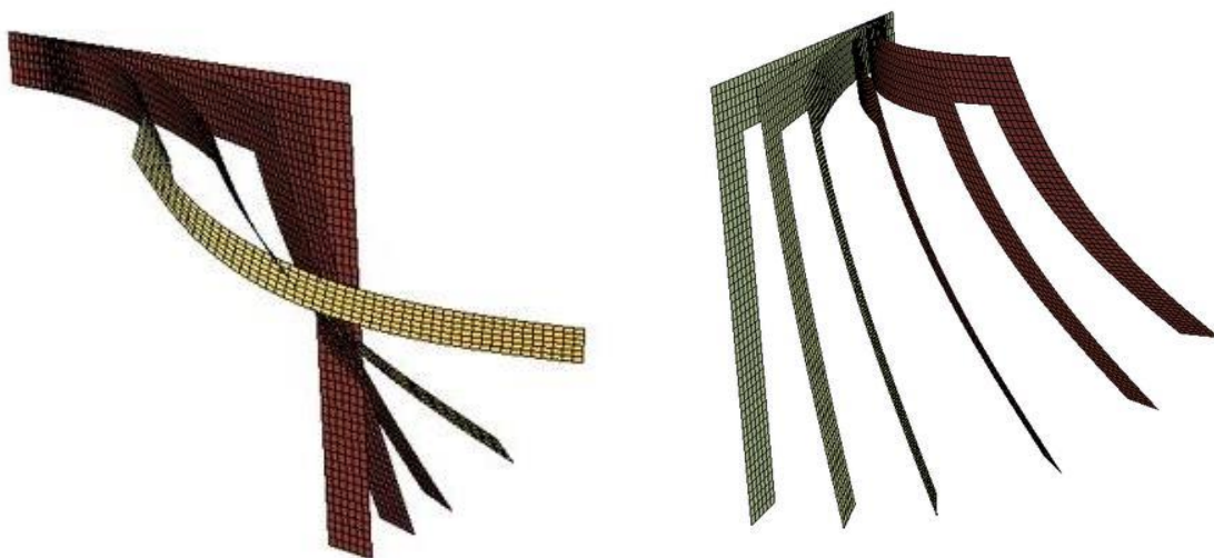
Figure 2.21: L-shaped plate: deformed finite element configurations; a) "tensile" force and b) "compressive" force.
