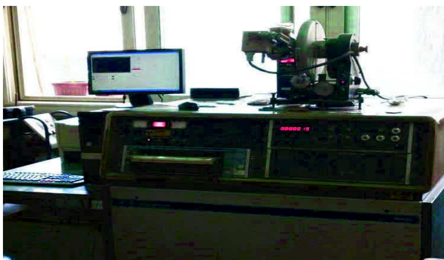
Fig. 5: Philips PW 1730 X-ray diffractometer used in the study.
