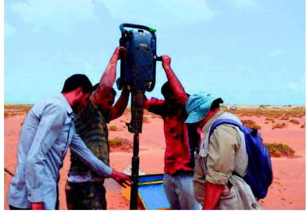
Fig. 40: Photo core dug using Cobra instrument.
