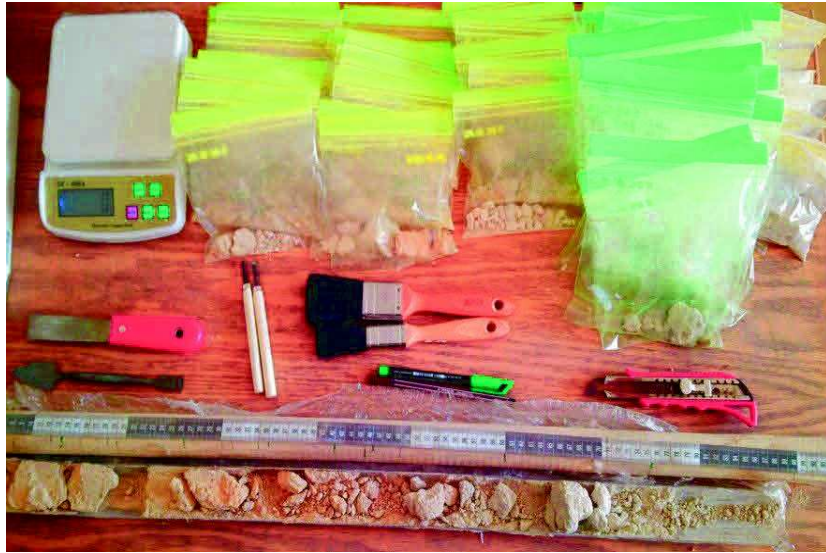
Fig. 3: Collected samples in this study of 25 grams for grain size and X-ray diffraction and totally organic and inorganic measurements
