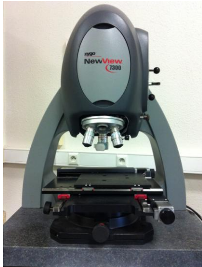
Figure 1: Optical interferometer Zygo NewView 7300 and Optical path of Mirau objective.
