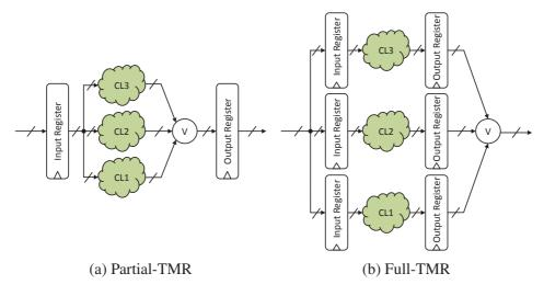
Fig. 2.13: Triple Modular Redundancy
