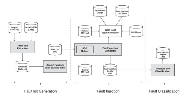
Fig. 2.17: Fault Injection Flow
