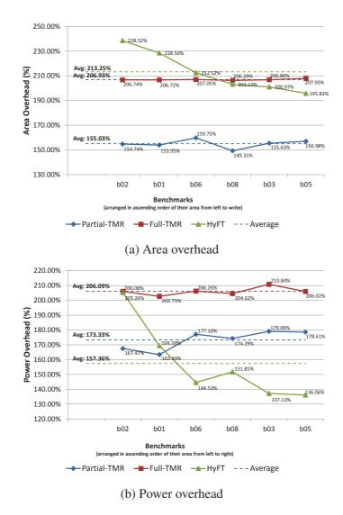
Fig. 2.19: Impact of CL blocks size on area and power overheads
