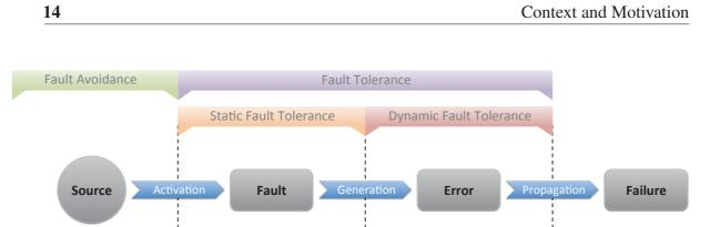
Fig. 1.4: Reliability improvement approaches across fault-failure life cycle [17]
