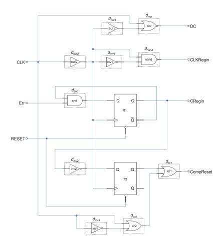
Fig. 4.8: HyFT-2b Control Logic submodule1
