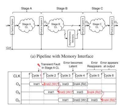
(b) Time plot of transient error propagation in Pipeline with Memory Interface
