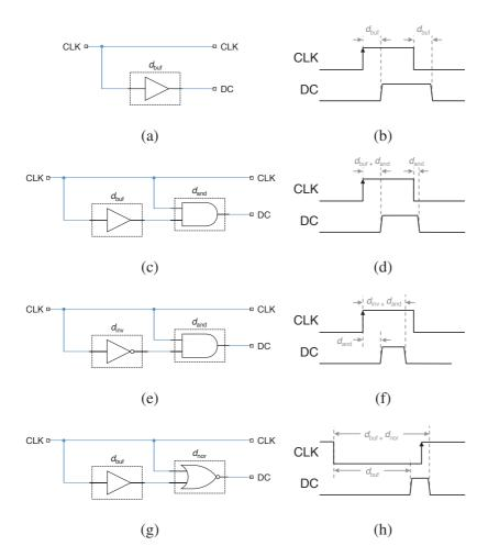
Fig. 4.1: Comparison-window Generation Circuits and delays
