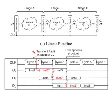
(b) Time plot of transient error propagation in Linear Pipeline
