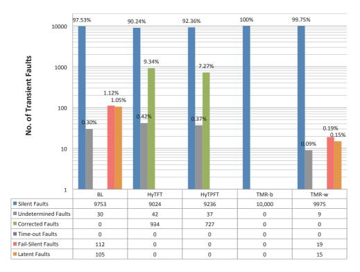
Fig. 3.18: Transient fault injection results
