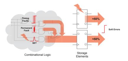
Fig. 1.5: Error occurrences in combinational logic and storage elements
