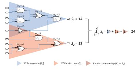
Fig. 5.6: Cumulative weight calculation of an example circuit
