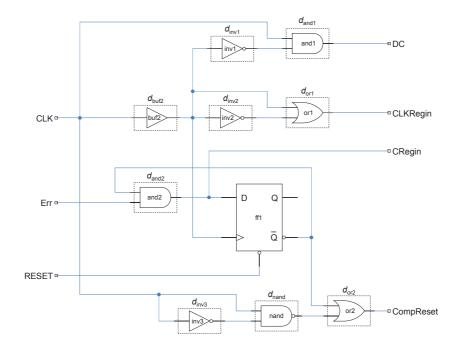
Fig. 4.6: HyFT-2a Control Logic submodule1
