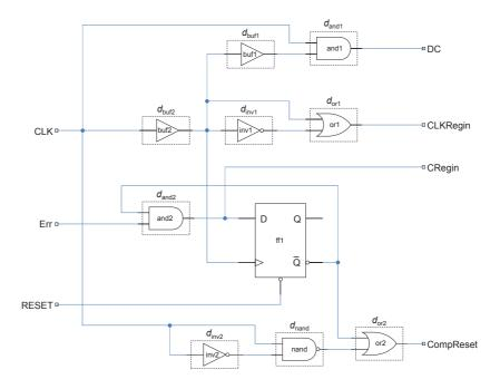
Fig. 4.4: HyFT-1b Control Logic submodule1
