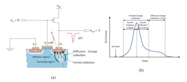
Fig. 1.3: Single Event Effect Mechanism [9]
