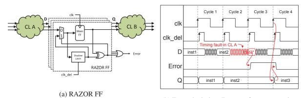
(b) Example timing diagram of error correction
