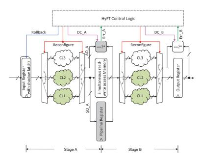
Fig. 3.11: HyFT hardening of pipeline stage with synchronous simultaneous read-write access memory.
