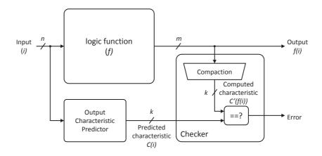
Fig. 2.7: General architecture of Error Detection with Codes [63]
