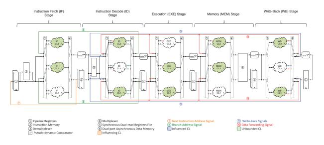
Fig. 3.14: HyTPFT Microprocessor
