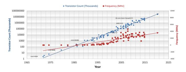
Fig. 1.2: Transistor count and clock frequency scaling trend over years [77]
