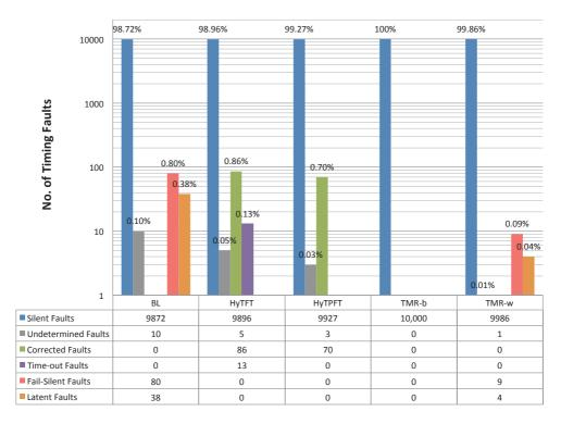
Fig. 3.20: Timing fault injection results
