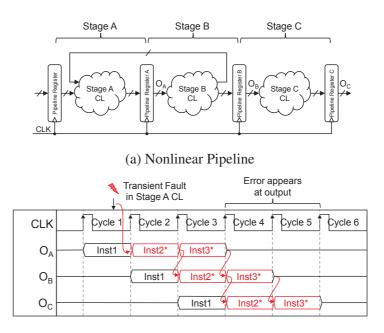
(b) Time plot of transient error propagation in Nonlinear Pipeline
