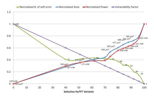
Fig. 5.7: Selective HyTFT cost versus soft-error (of CL block extracted form b05)
