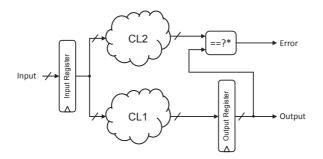
Fig. 2.6: Error detection architecture using the pseudo-dynamic comparator [93]
