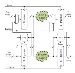
Fig. 2.12: CPipe Architecture [89]
