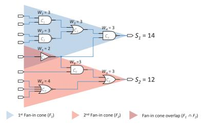
Fig. 5.1: Application of the output susceptibility analysis on an example circuit
