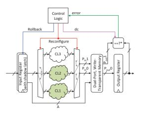
Fig. 3.10: HyFT hardening of pipeline stage with asynchronous non-concurrent read-write access memory.
