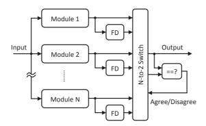
Fig. 2.9: Principle of PaS redundancy
