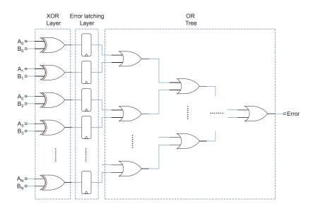
Fig. 2.3: An static comparator with Error Latching mechanism moved upstream
