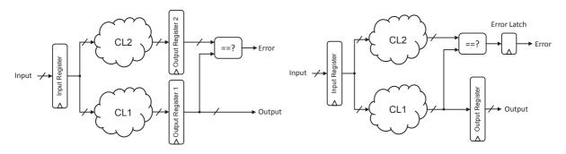
(a) Comparator placed after output register
