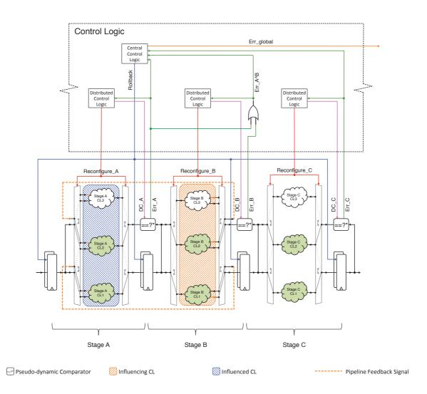
Fig. 3.9: Error detection and reconfiguration scheme in non-linear pipeline
