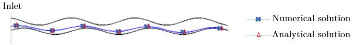
Figure 3.7: Comparison between particle trajectories in the same channel as found in the numerical simulation and as predicted by the analytical model
