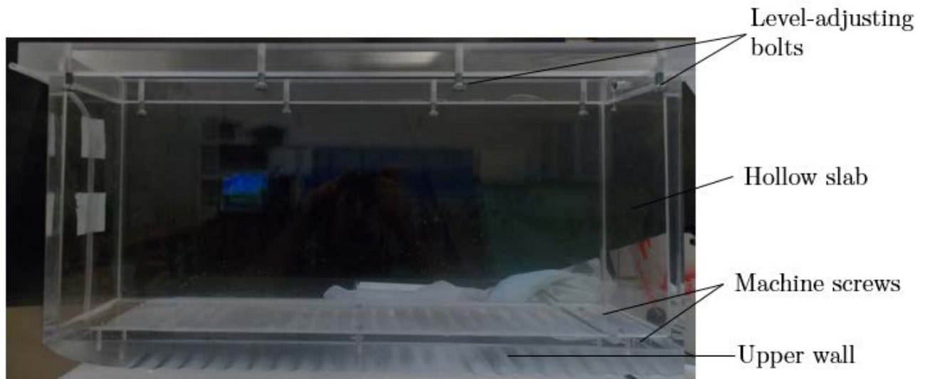
Figure 4.6: The hollow slab holding the upper wall and the bolts used to raise and lower the slab.
