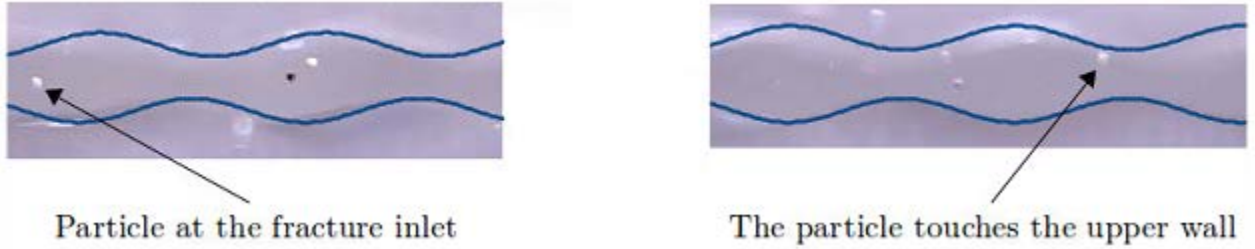
Figure 4.23: Particle with Z_p^0 \simeq 0 traveling through the fracture until it touches the upper wall.
