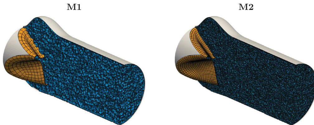
Figure 4.4: Computational zone of interest composed of the valve solid mesh and the aortic fluid mesh. Two levels of mesh are considered, the coarse mesh M_1 and the fine mesh M_2 .
