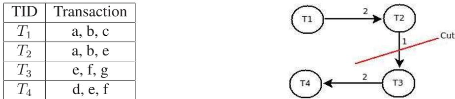
Figure 3.1 – Transactions of a database (left) & Graph representation of the database (right)
