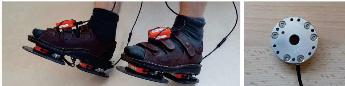
(b) Shoes equipped with inertial measurement units and force-torque sensors.
