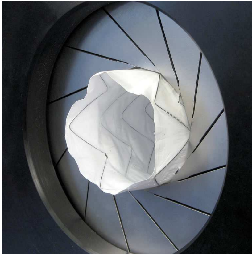
Fig: 21 This machine is able to measure the radial fore produced during the eccentric expansion of the stent (Photo MSI Company)
