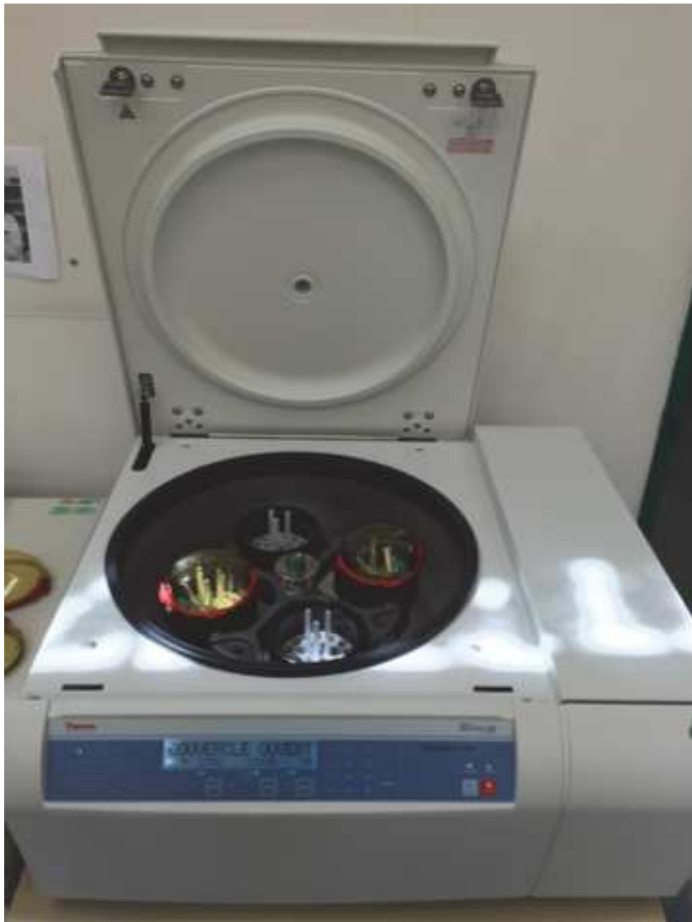
Fig. 27 The centrifuge machine used in our experiments to produce white stiff clot from platelet rich plasma. Tubes containing whole blood were centrifuged at 350g for 10 minutes at 22°C.
