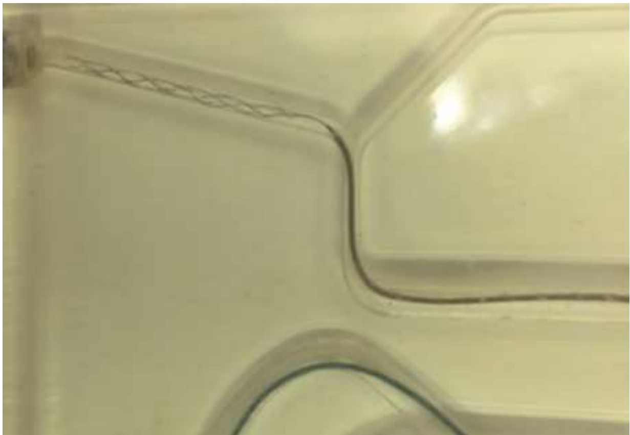
Fig 25. In this figure a stent retriever is placed at the level of the middle cerebral artery of the phantom to perform a “Retrieving test”.
