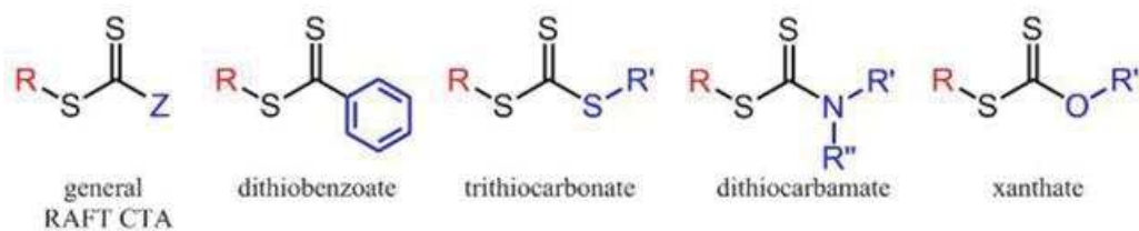
Figure 1.3.4. Generic chemical structures of chain transfer agents (CTAs) used in RAFT polymerization. 13,27
