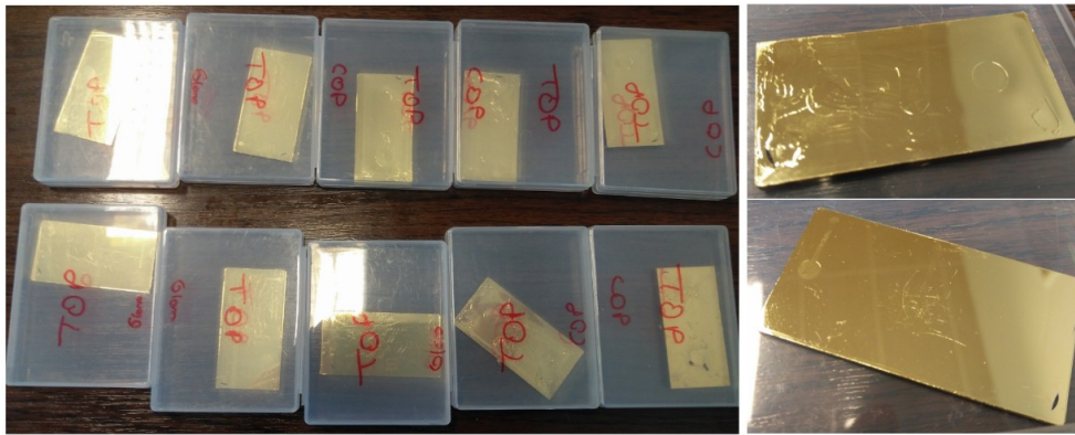
Figure 94 : Results of the gold deposition on top of COP and glass slides (left), with a COP slide (right-top) and glass slide (right-bottom)
