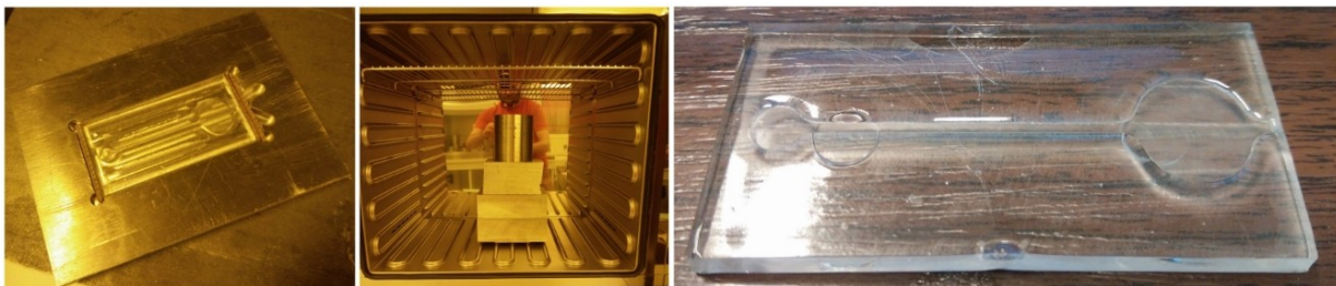
Figure 83 : From left to right, aluminum milled hot embossing imprint, hot embossing process before start & a hot embossed COP fluidic channel
