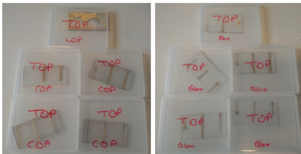
Figure 95 : Results of the lift-off and scalpel grinding operations on COP slides (left) and glass slides (right)
