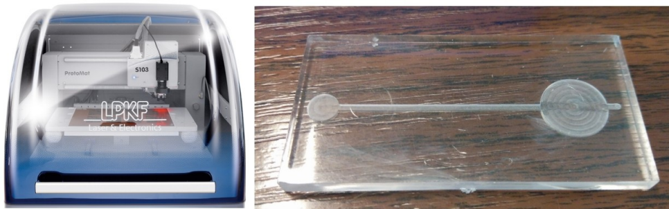
Figure 81 : LPKF S103 CNC (left) and micro-machined COP fluidic channel (right)
