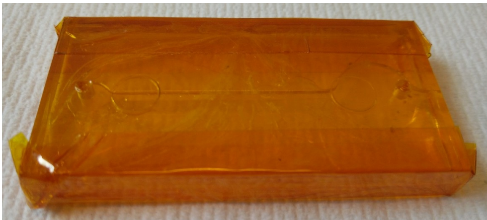
Figure 109 : Kapton (polyimide) film coated COP chip
