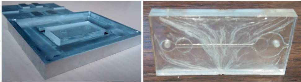
Figure 89 : COP thermal bonding support holding a COP chip before bonding (left) and a bonded chip (right)
