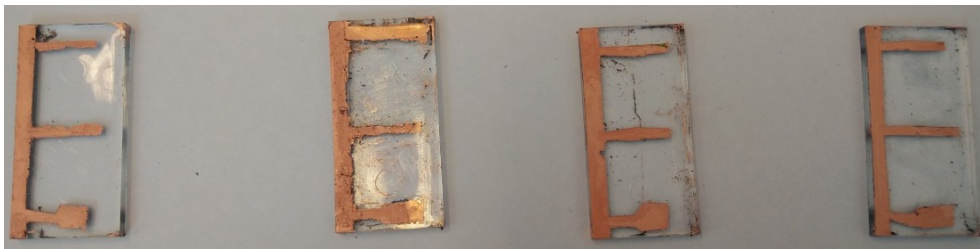
Figure 96 : COP slides after metallization with copper
