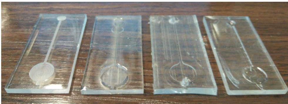
Figure 86 : From left to right, micro-machined COP, hot-embossed COP, molded PDMS & COP laser engraved fluidic chip
