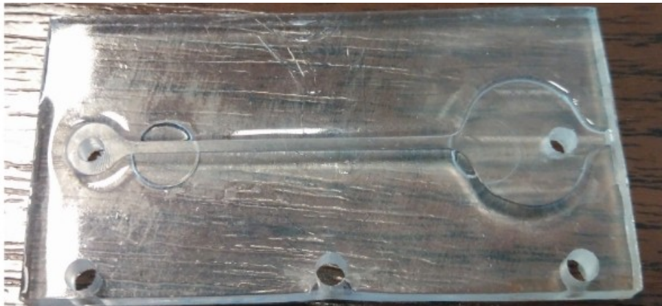
Figure 107 : COP fluidic channel after injection and electrodes access holes drilled through it
