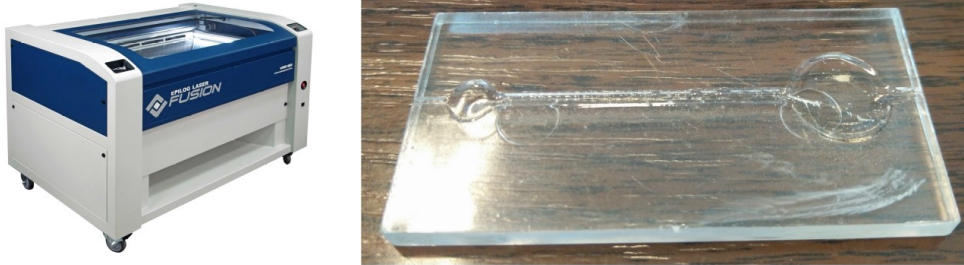
Figure 82 : EPILOG fusion CO2 cutting laser (left) and laser engraved COP fluidic channel (right)
