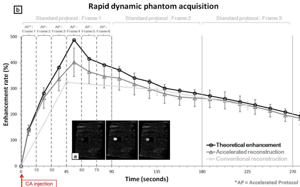
**Figure 7:** Data acquired on a dynamic breast lesion phantom with the modified VIBRANT sequence. a) Image reconstructions with a compressed-sensing based algorithm – Contrast uptake visual follow-up on one slice centered in the phantom b) Contrast uptake curves – error bars represent the standard deviation in the enhancement ROI. Temporal resolutions were respectively 90 sec and 15 sec for conventional and accelerated reconstructions
