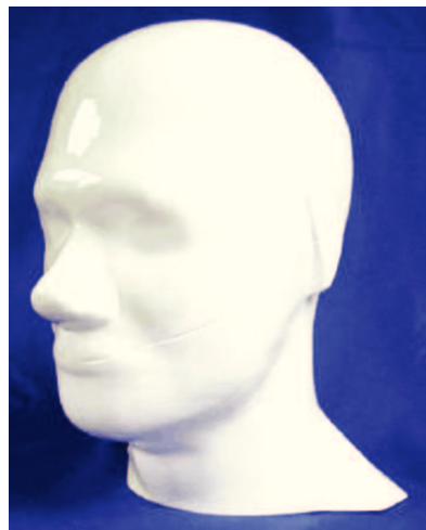
Figure 2.11: International reference phantom: Specific Anthropomorphic Mannequin (SAM)
