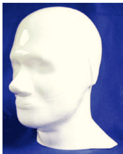
Figure 2.11: International reference phantom: Specific Anthropomorphic Mannequin (SAM)
