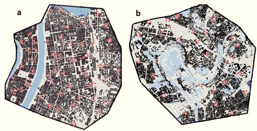
Figure 3.12: Network models of macro cell deployments: macro 3G network in urban (a) and suburban (b) area
