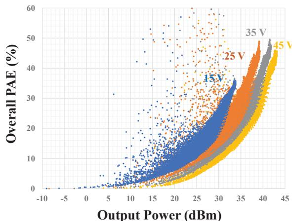
Figure III.47: (a) Measured overall PAE at 19 dBm input power LO at  $f_c = 2.2$  GHz.
