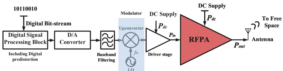
Figure I.2: General Architecture of RF Power Transmitter Chain
