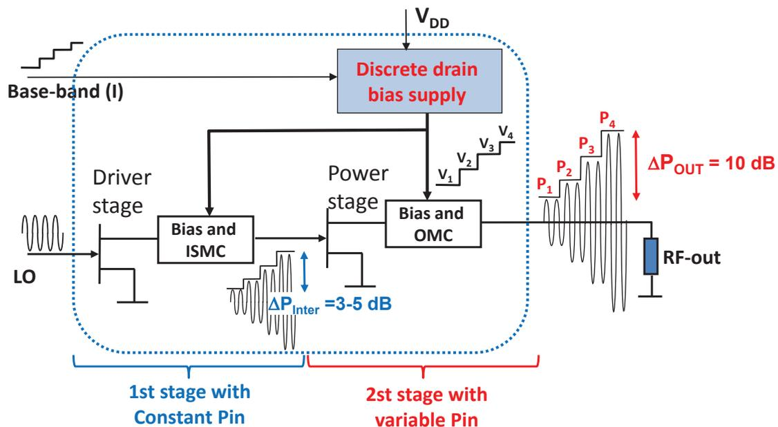
Figure III.3: Working principle of the Vector Power Modulator.
