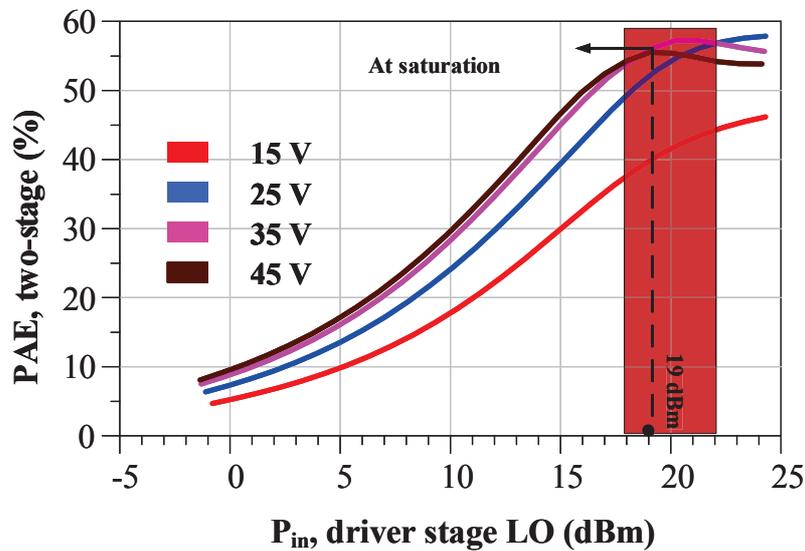
Figure III.34: PAE as a function of input power LO of driver stage for the overall two-stage power modulator circuit at 2.5 GHz.
