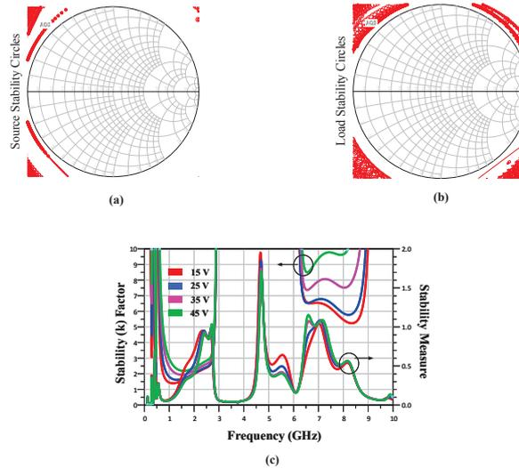
Figure III.25: Unconditional Stability after the implementation of the stability network for the driver-stage (a) Source Stability Circles (b) Load Stability Circles and (c) Stability Factor,  $k$  and Stability Measure,  $\Delta$  .
