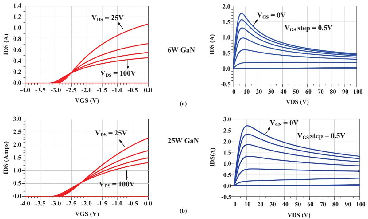
Figure I.22: DC-IV characteristics: (a) Cree CGHV1F006S (b) CGHV1F0025S.
