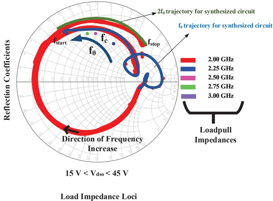
Figure III.29: Optimum load impedance loci of the driver stage from loadpull and from the synthesized circuit at reference plane  $\Delta P_1$  of fig. III.28. The impedance indicates clearly the  $2f_0$  of the synthesized circuit is not well matched and is close to the unfavourable region.
