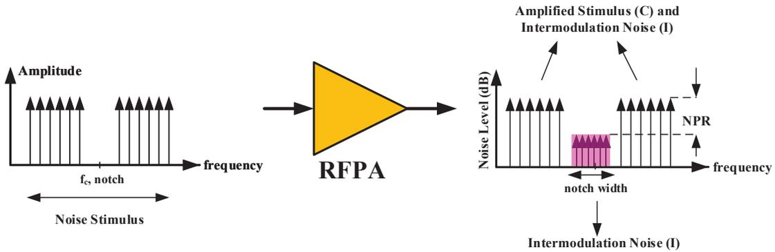
Figure II.9: A digital NPR test stimulus with white noise source connected in cascade with a bandpass filter and a notch filter. The notch depth can be measured with a Spectrum Analyzer.
