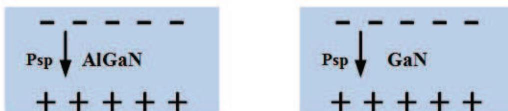
Figure I.19: Spontaneous polarization induced surface charges in the AlGaIn and GaN structure.([14])
