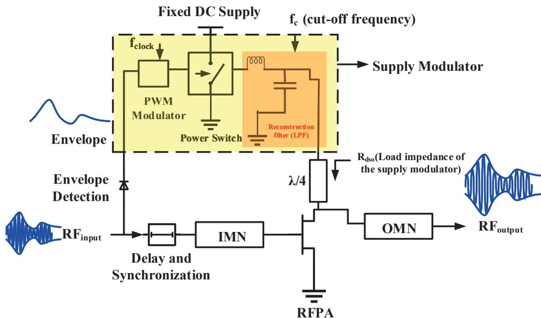
Figure II.23: Simplified architecture of Envelope Tracking amplifier
