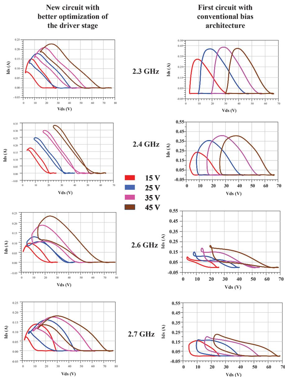
Figure IV.12: Comparison of the driver stage current source dynamic loadlines at different frequencies for  $P_{in}=22$  dBm (new circuit),  $P_{in}=19$  dBm (first circuit) and  $15\text{ V} < V_{dso} < 45\text{ V}$ .
