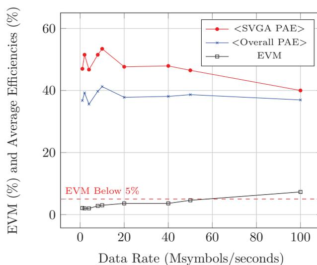
Figure III.49: Measured overall average PAE, EVM and PAE of the SVG circuit at 19 dBm average input power LO at 2.2 GHz.
