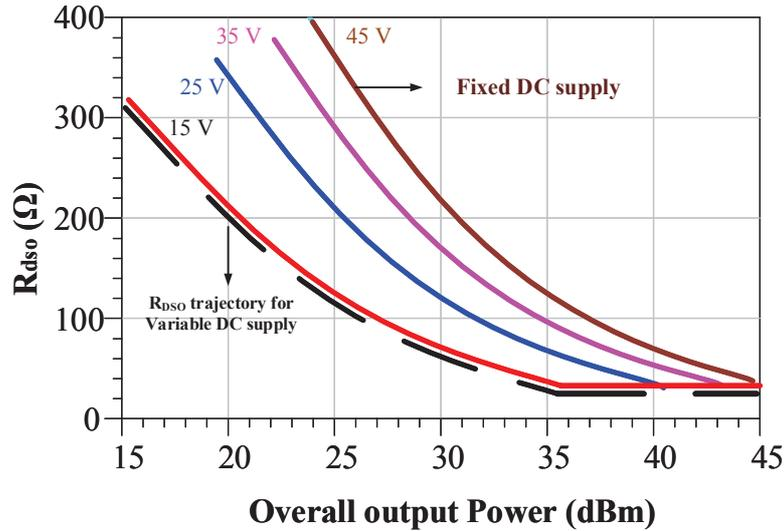
Figure II.24: Simulated values of drain resistance  $R_{dso}$  as a function of output power.
