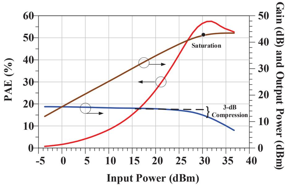
Figure I.10: Power characteristics of a conventional GaN based RF power amplifier
