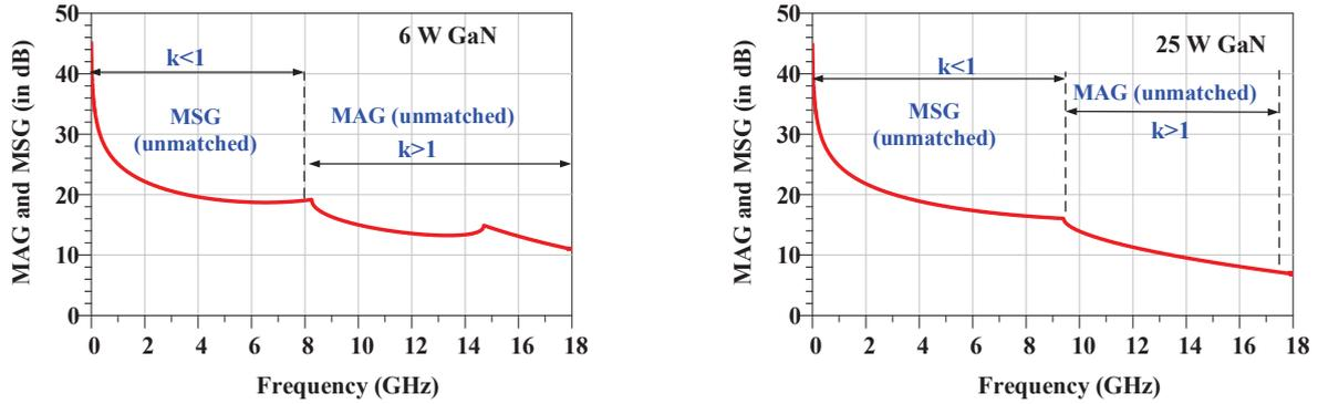
Figure I.23: Simulated MAG and MSG capabilities of the 6 W (left) and 25 W (right) packaged GaN transistor alone.
