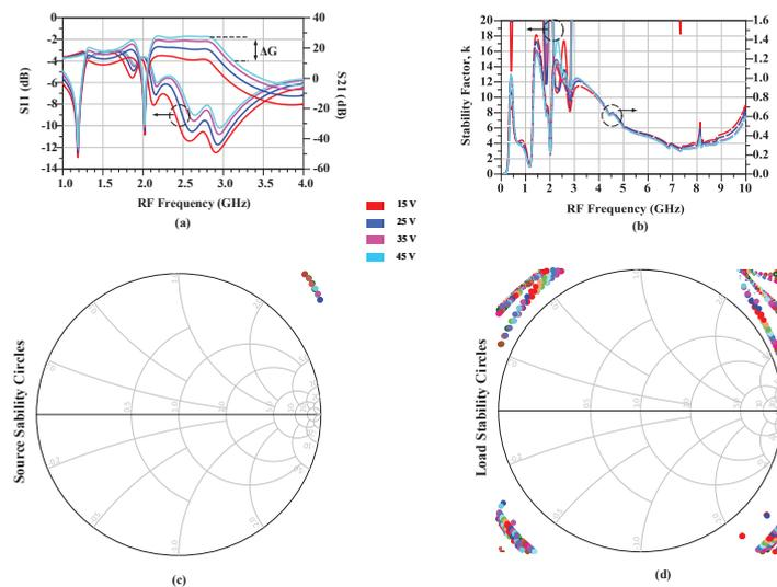
Figure IV.4: S-parameters of the new vector power modulator circuit (a)  $S_{11}$  and  $S_{21}$  (b) Stability factor ,  $k$  and stability measure (c) Source stability circles and (d) Load stability circles .
