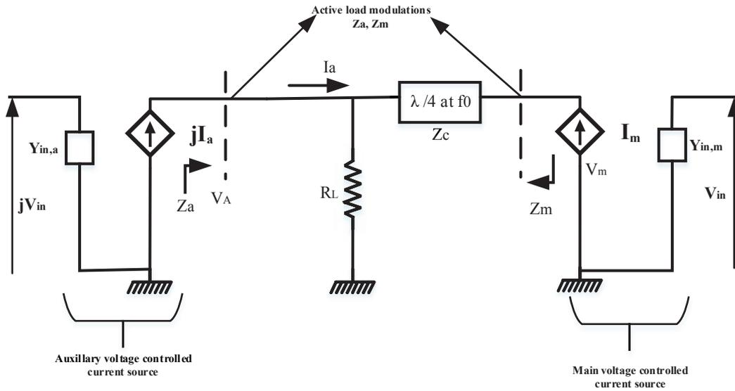
Figure II.15: Principle of Active Load Pull in Doherty Technique.
