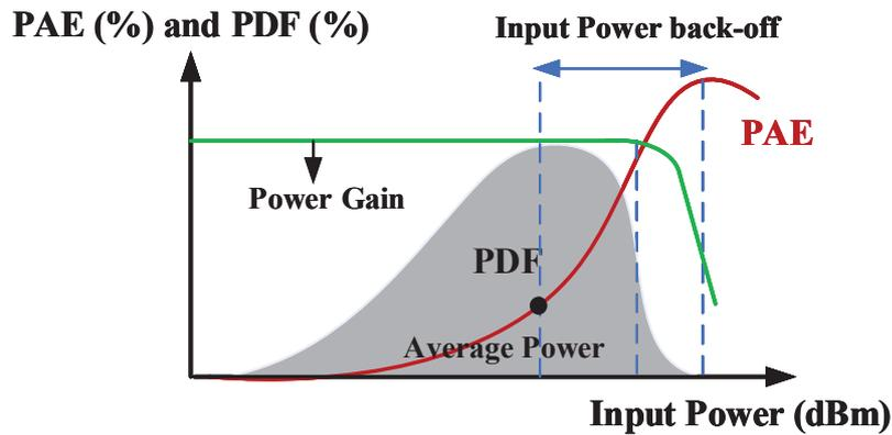
Figure II.5: Typical RFPA efficiency with respect to input power. Probability density function for a high PAPR signal at an average output power level example is illustrated.
