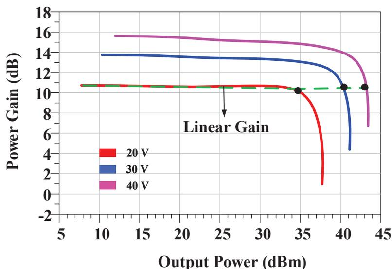
Figure II.22: Simulated CW gain characteristics as a function of drain output power with the optimum trajectory corresponding to linear gain at different drain voltages.
