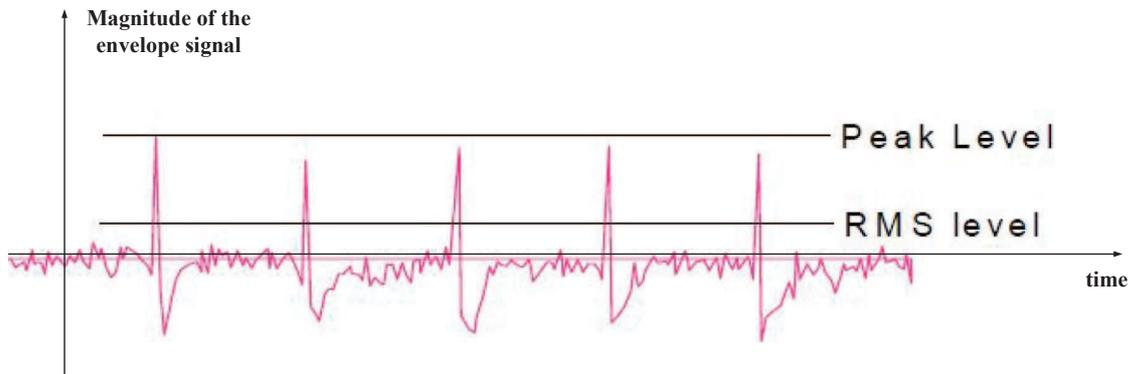
Figure II.3: Crest Factor Representation for Complex Modulated Signal
