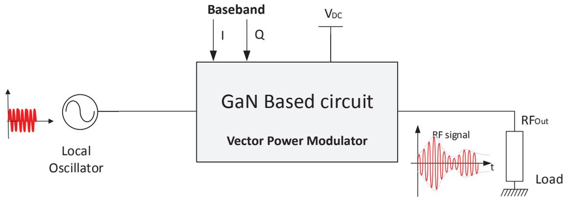
Figure III.2: Proposed GaN based Vector Power Modulator.
