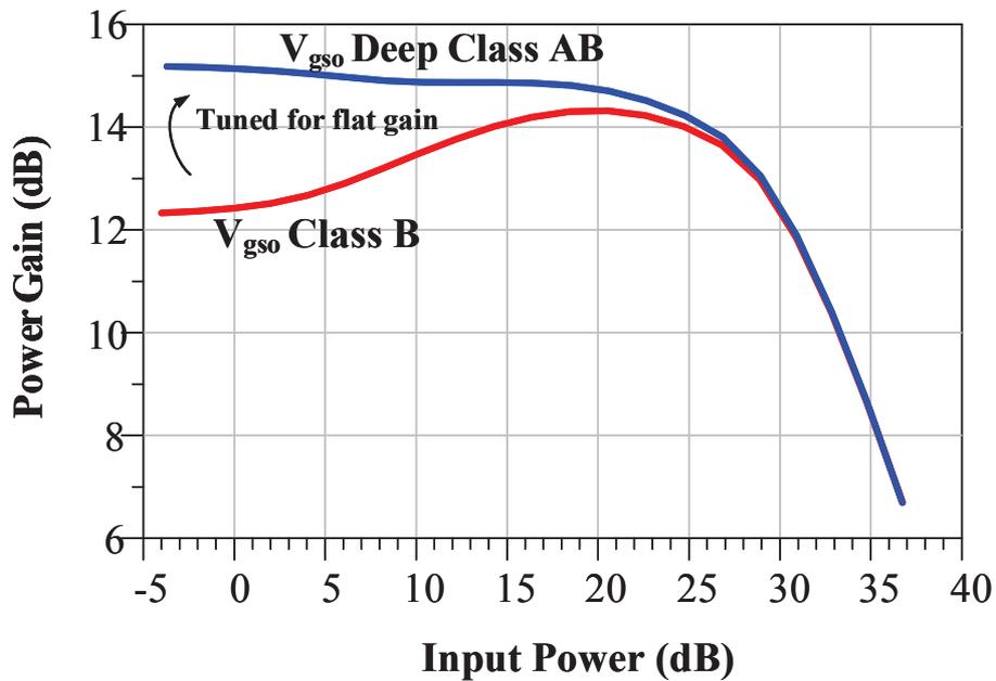
Figure I.9: Gain characteristics of a conventional RF power amplifier
