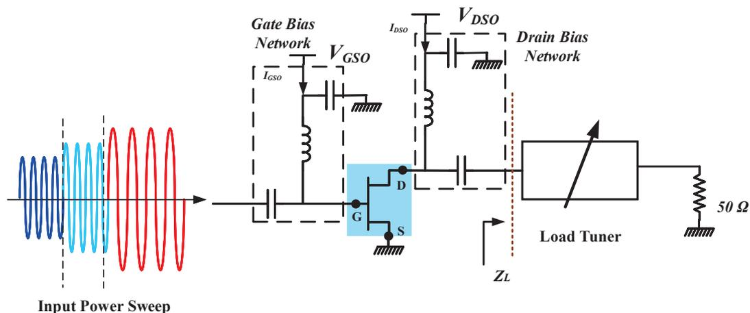
Figure II.11: General schematic of an RFPA with a load tuner demonstrating load variation for three different input power levels.
