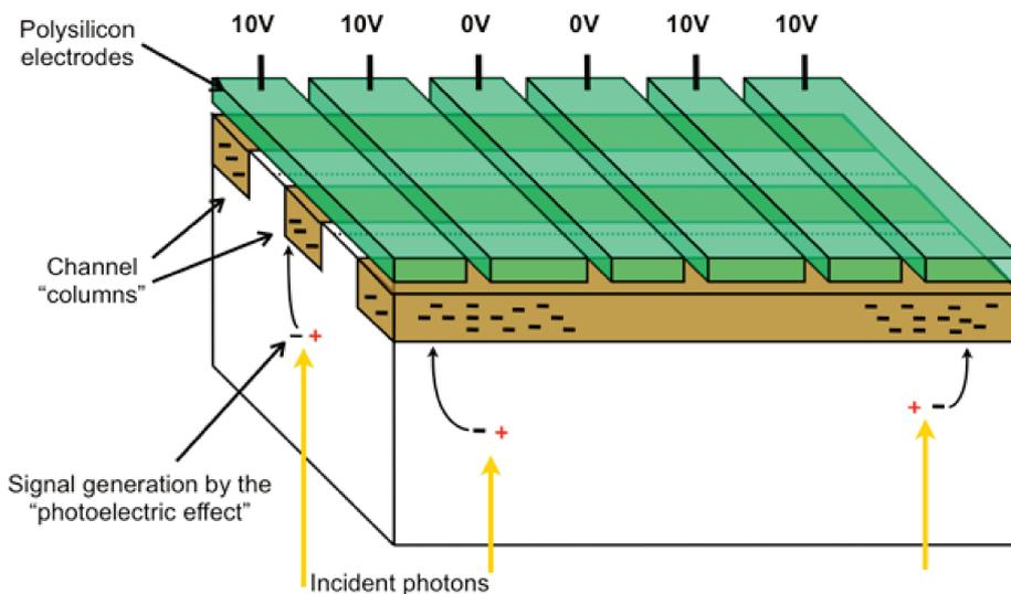
Figure 2.16 – Scheme of a CCD. Photons are converted into electrons via the photoelectric effect and being attracted to the potential wells under electrodes with positive voltage applied. (Copyright: Oxford University Press).
