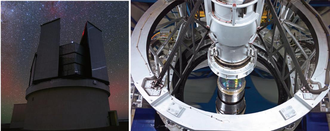
Figure 2.13 – **Left:** The VISTA telescope in Paranal. Image Credit: Y. Beletsky (LCO)/ESO. **Right:** Image of the 4.1 metre mirror of the telescope. The entrance lens of VIRCAM (VISTA InfraRed CAMera), the giant infrared camera, is visible at the centre, under the structure that supports the secondary mirror. Credit: ESO.
