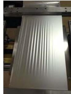
Figure 1.2: Instability in metal film under uni-axial tension
