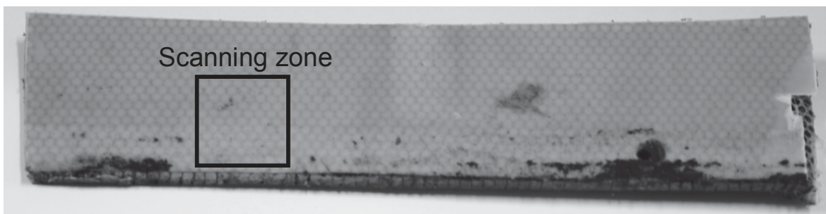
Fig. B.2 The photo shows a composite synthetic material, the black square marks a scanning area.
