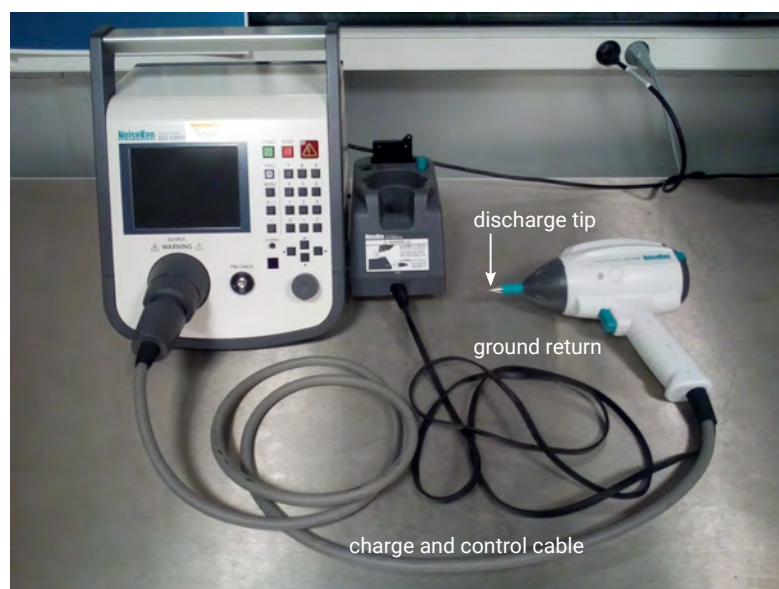
Figure 1.11: Picture of an ESD gun IEC 61000-4-2 compliant
