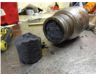
Figure 3: Sulphide scale collected from the Elgin well
