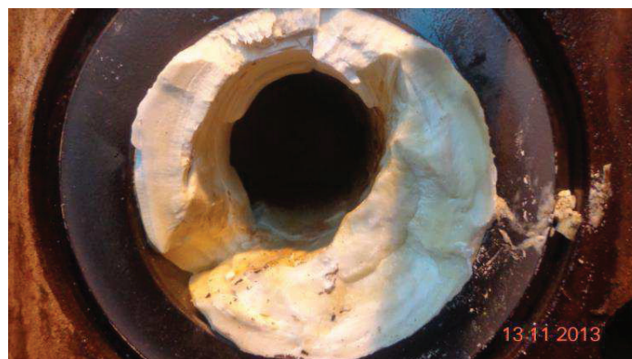
Figure 1: Scale formation in pipeline. The combined effect of high pressure and temperature with the high concentration of scale precursors dramatically decrease the efficiency of oil and gas production.
