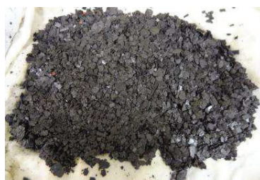
Figure 3: Sulphide scale collected from the Elgin well
