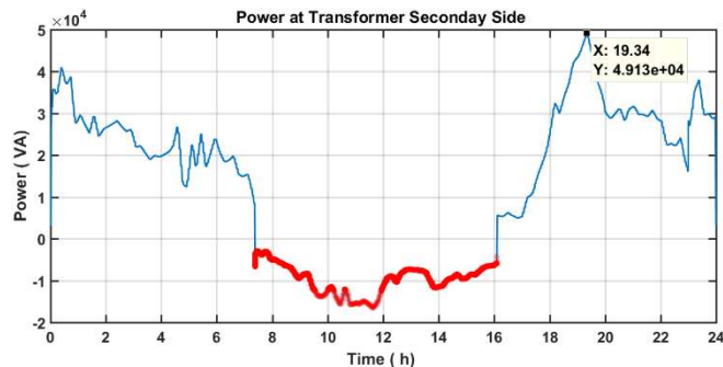
Fig. 4.25 Power at transformer (Phase1 + Phase 2)
