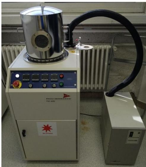
Figure 2.19 Photo of Parylene C vacuum deposition device (PDS 2010, Specialty Coating Systems, KISCO) installed in ENS laboratory.
