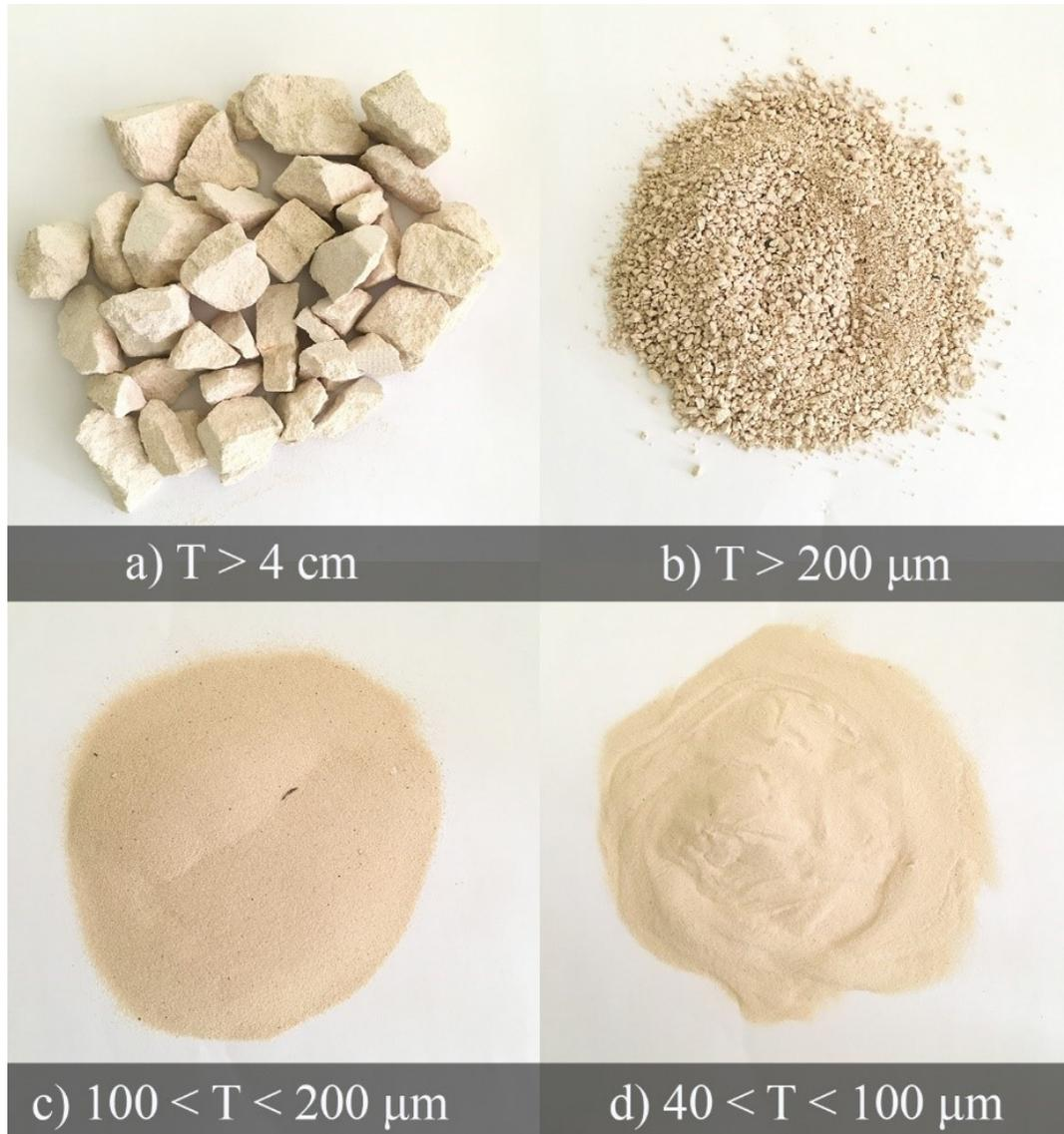
Figure 2. 7: Different levels of grinding of Lavoux limestone in order to separate oolites from other components.
