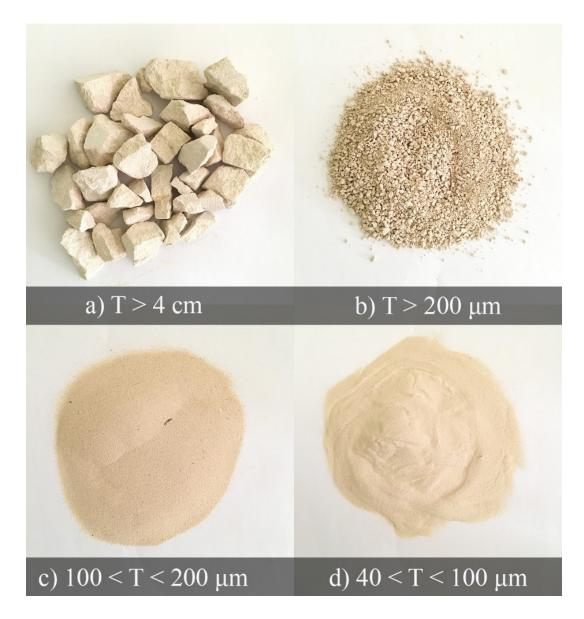
Figure 2. 7: Different levels of grinfing of Lavoux limestone in order to separate oolites from other components.
