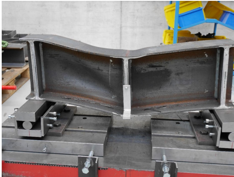
Figure 4-34: Failure of test IPE 270_S355_L810 by local buckling of the web
