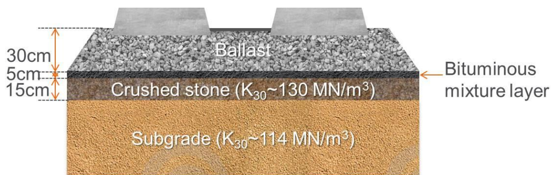
Figure 1.16. Schematic cross section of a typical Japanese HSL track with bituminous sub-ballast layer (adapted from (Rose et al., 2011))
