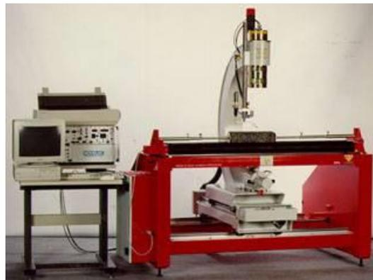
**Figure 1.10.** Vertical gamma-densitometer bench (Dubois et al., 2010)
