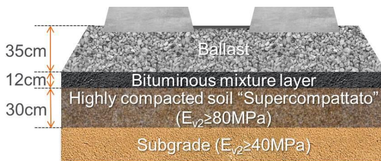
Figure 1.14. Schematic cross section of a typical Italian HSL track with bituminous sub-ballast layer (adapted from (Rose et al., 2011))
