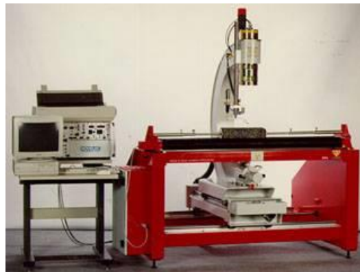
Figure 1.10. Vertical gamma-densitometer bench (Dubois et al., 2010)
