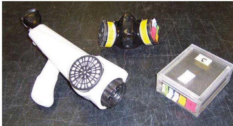
Figure 2.12 – Field olfactometers (from left to right): Nasal Ranger ® , Mask Scentometer and Box Scentometer.
