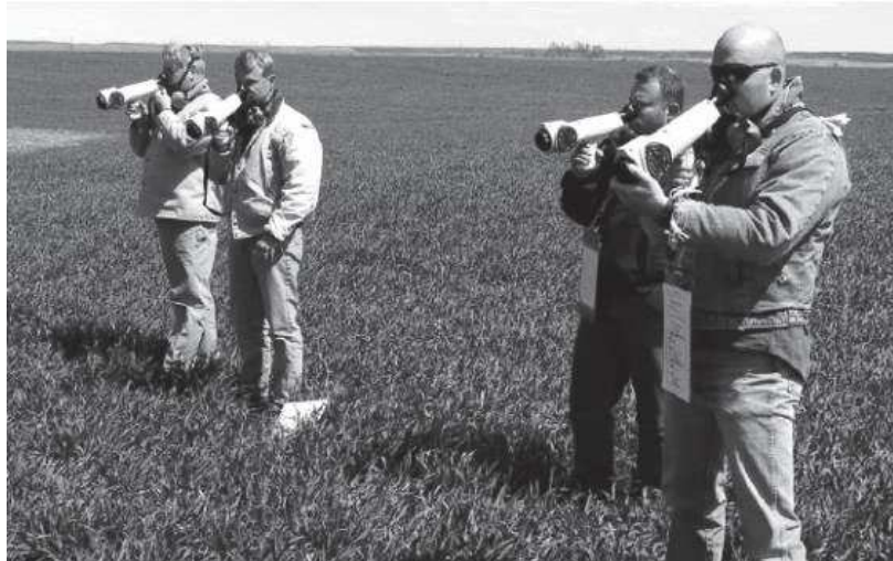
Figure 2.16 – Nasal Ranger® Field Olfactometer being used in field observations.
