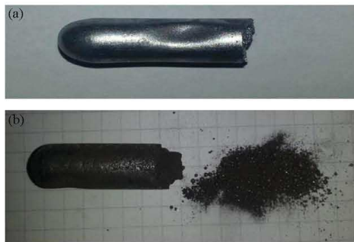
Figure 6. Macroscopic observation of (a) undoped ZnSb sample and (b) 1 at% B-doped ZnSb ingot.
