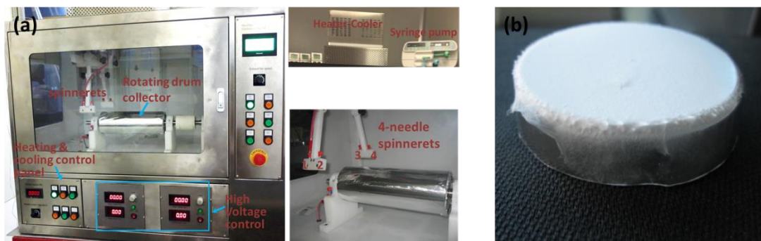
Figure 2.16 Photos of (a) electrospinning set up installed in the ENS laboratory (b) fiber sample deposition.
