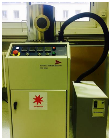
Figure 2.10 Photo of parylene deposition system (SCS Instruments) installed in the ENS laboratory
