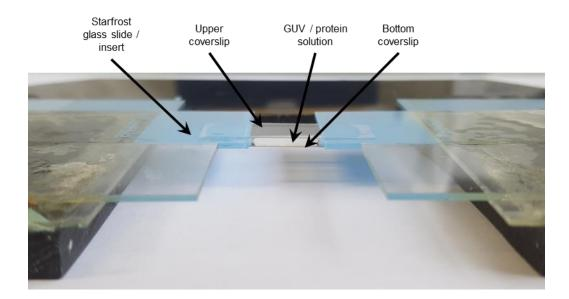
**Figure 3.10: Experimental chamber for tube pulling experiments.** This hand-made chamber has the particularity to be opened on the side allowing the insertion of the micropipette.
