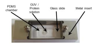
**Figure 3.9: Hand-made PDMS chamber in metal insert.** Studies of protein recruitment to GUVs of different compositions were always performed with this device.
