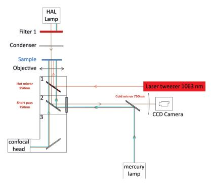
**Figure 3.6: Schematic of the microscope experimental setup.** The setup developed in the lab by D. Guet is composed of a confocal head which uses visible light (rainbow beam with simple arrow, port n°3), an optical tweezer which functions at 1063 nm (red beam, port n°1), a bright field visualization module which uses near infrared light (brown beam, port n°2) and finally epifluorescence mode (rainbow beam with triple arrows, port n°2). From (Guet, 2012).
