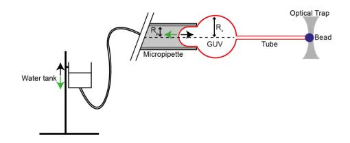
**Figure 3.11: Tube pulling experimental setup.** A biotinylated lipid-containing GUV is aspirated into a micropipette connected to a water tank of adjustable height which allows the control of membrane tension. A streptavidin coated bead is immobilized using an optical trap and a membrane tube is formed by the biotin-streptavidin interaction. Lowering of the water tank will lead to an increase in membrane tension and consequently a decrease of the tube radius. (Not to scale).
