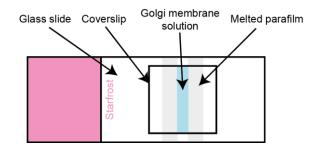
**Figure 3.I3: Experimental chamber for Golgi membranes studies.** A glass coverslip is fixed to a Starfrost glass slide with melted parafilm in between. The parafilm acts as a spacer and also allows isolation of the chamber. This hand-made chamber has the advantage of working with small volumes (5 μL).
