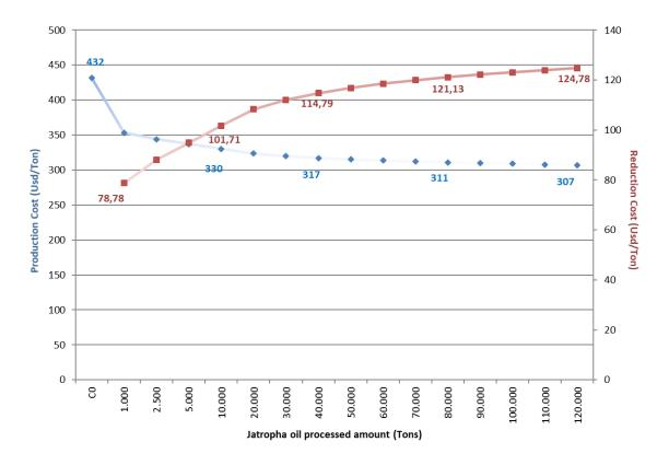
Figure 6. 8. Operational cost for the jatropha oil transformation (b=1) with technology d=1 and production capacity g=1 (40,000 tons/year) at principal plants
