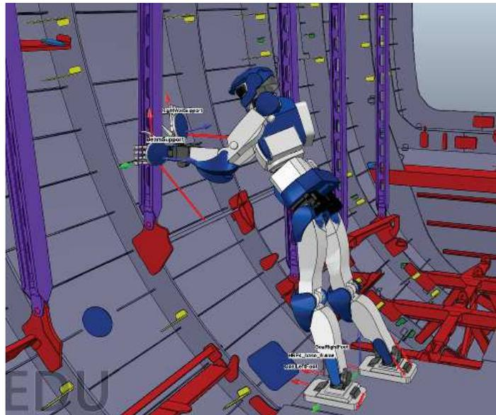
Figure 5.2 HRP-4 applying a desired force on a contact point with its right hand.
