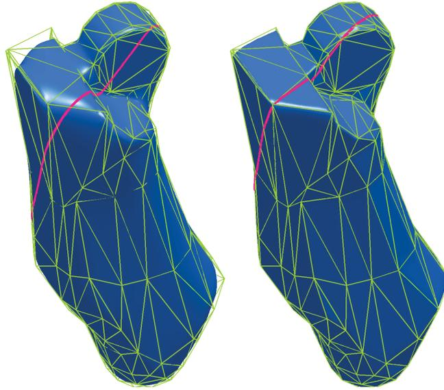
Figure 5.8 Catmull-Clark Surfaces (in blue) approximating the mesh of a link on HRP-2 (in green)
