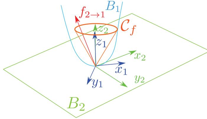
Figure 2.4 Punctual unilateral stability contact with friction
