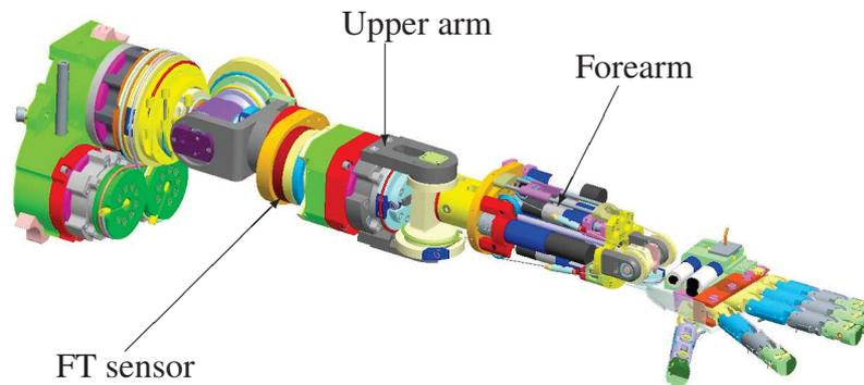
Figure 6.4 CAD drawing of the iCub arm used in the experiments. The six-axis F/T sensor used for validation is visible in the middle of the upper arm link.
