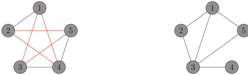
Figure 2.1: On the left a graph admitting an Hamiltonian Cycle (positive instance), on the right a graph without Hamiltonian Cycle (negative instance).
