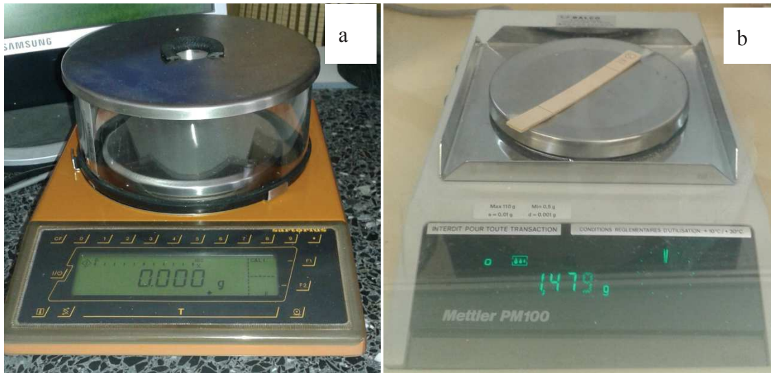
Fig. A.12. Balances for (a) oven dried specimens and (b) stabilized specimens measurements
