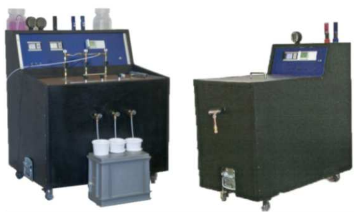
Fig. B.6. Reactor for hydrothermal treatment developed by Biel University
