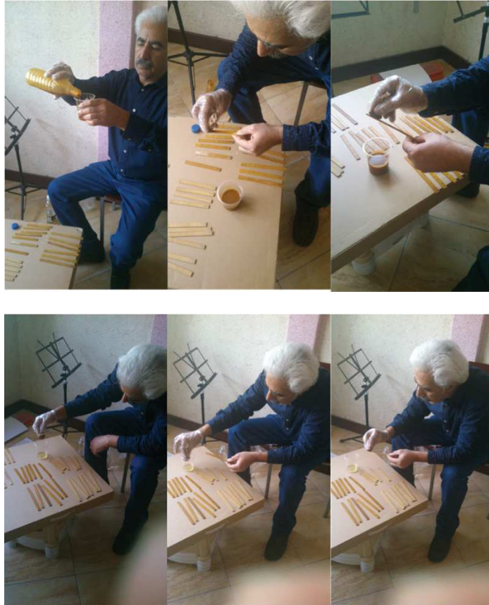
Fig. C.1 The steps of workshop varnishing procedure for all the specimens varnished by a professional instrument maker in Iran. (a), preparing cotton for varnishing (b), applying Shellac (c), Polyester (d) and Sandarac (e) with a professional instrument maker in Iran.
