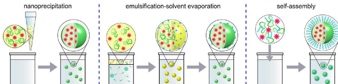
Figure 1.17. Techniques used for the preparation of dye loaded NPs from preformed polymers. Hydrophobic polymer segments are shown in green, hydrophilic ones in blue, organic solvent in yellow. Adopted from ref. [71]
