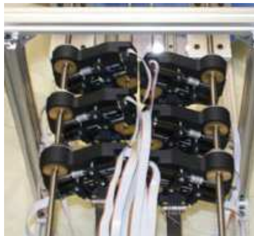
Figure 2.3 – RTC equipped with two three-tubes arms and an actuation serial unit without coupling [Burgner et al., 2011] [Burgner et al., 2014].
