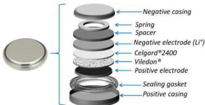
Figure 2-6. Exploded view of 2032 coin cells components in half-cell configuration versus metallic lithium, reproduced from [255].
