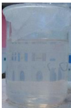
Figure 3-4. Picture of a Li,Mn,Si gel catalyzed by acetic acid with medium precursors' concentration condition (see Table 3-2).
