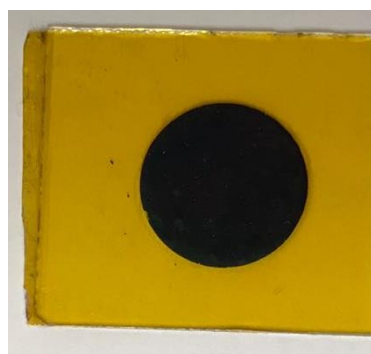
Figure 2-5. Picture of a positive electrode stuck onto a microscope glass slice for the purpose of ex-situ XRD measurements.
