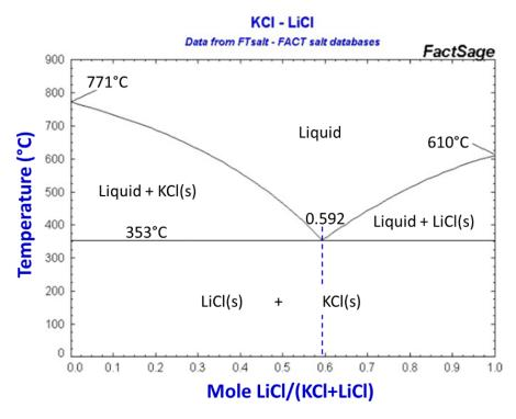
Figure 4-5. Binary diagram of LiCl-KCl generated and adapted from the software FactSage [281].
