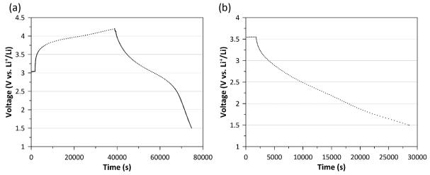
Figure 4-45. (a) First galvanostatic cycle of Li<sub>2</sub>MnSiO<sub>4</sub>/C positive electrode charged to 4.2V and discharged to 1.5V at C/20 (1C=333mA.g<sup>-1</sup>) and (b) residual discharge of  $Mg_{1-x}MnSiO_4/C$  positive electrode to 1.5V at C/10 (1C=174mA.g<sup>-1</sup>), tested at CEA. Discharge capacities are used to define the nominal capacity of the battery at the beginning of testing.
