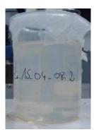
Figure 3-5. Picture of a Li,Mn,Si gel using the intermediate P123 content condition.
