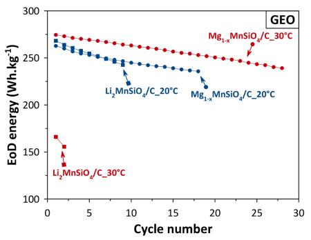
Figure 4-49. Evolution of End of Discharge energy of  $Li_2MnSiO_4/C$  (squares) and  $Mg_{1-x}MnSiO_4/C$  (circles) based coin cells at 20°C (blue) and 30°C (red) as function of cycle number, for GEO cycling conditions.
