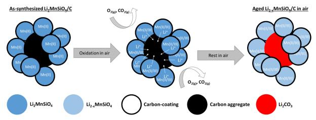
Figure 3-46. Scheme illustrating the main mechanism of the reactivity of Li<sub>2</sub>MnSiO<sub>4</sub>/C with air.
