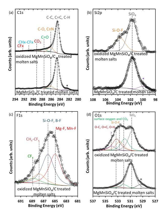
Figure 4-30. XPS C1s (a), Si2p (b), F1s (c) and O1s (d) normalized spectra of MgMnSiO<sub>4</sub>/C treated in molten salts and oxidized MgMnSiO<sub>4</sub>/C treated in molten salts. Calibration with Si2p component of SiO<sub>4</sub> at 101.7eV. The charge effect is represented by a component which is marked by a star "\*" on C1s, Si2p and O1s spectra of MgMnSiO<sub>4</sub>/C treated molten salts.
