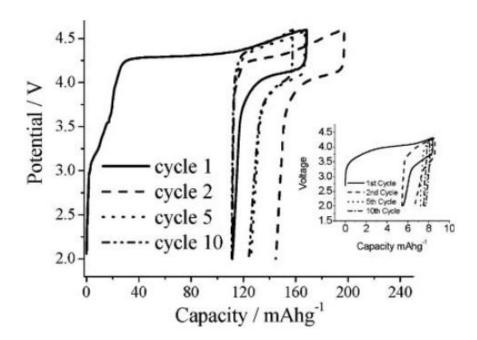
Figure 1-18. Variation of voltage with state of charge (Li content) on cycling the  $\beta_i$ -Li<sub>2</sub>CoSiO<sub>4</sub> polymorph carbon coated by the xerogel process at a rate of 10mA.g<sup>-1</sup>, from [100]. Inset shows performance of uncoated material.
