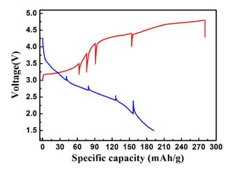
Figure 1-22. First galvanostatic cycle performed at 15mA.g<sup>-1</sup>, between 1.5V and 4.8 V, on Li<sub>2</sub>FeSiO<sub>4</sub>/C material, adapted from [136].
