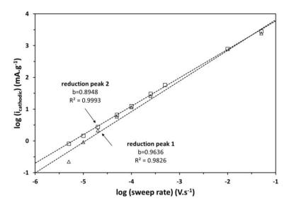
Figure 4-36. Evolution of reduction peaks current as a function of sweep rate for oxidized MgMnSiO<sub>4</sub>/C. The reduction peaks here correspond to those of Figure 4-35. The slop, b, of Equation 4-4 is indicated as well as the correlation coefficient,  $R^2$ .
