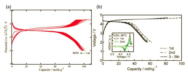
Figure 1-7. (a) Galvanostatic charge–discharge curves for  $Li_2FeP_2O_7$  positive electrode at C/20 [57], Galvanostatic voltage-composition curve of  $Li_2MnP_2O_7$  at a rate of C/50 obtained at 40°C, the corresponding dQ/dV plot is shown in inset [59].
