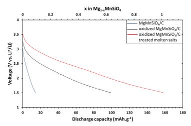
Figure 4-31. Direct galvanostatic discharge of MgMnSiO<sub>4</sub>/C (blue curve), oxidized MgMnSiO<sub>4</sub>/C treated in molten salts (black curve) and MgMnSiO<sub>4</sub>/C previously charged at 4.8V (blue curve) between 1.5V and 4.8V at C/20 (1C=313mAh. $g^{-1}$ ) and room temperature.
