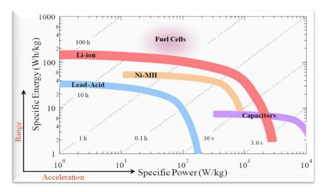
Figure 0-2. Ragone plot of electrochemical devices according to their specific energy ( $Wh.kg^{-1}$ ) and specific power ( $W.kg^{-1}$ ), adapted from [9].
