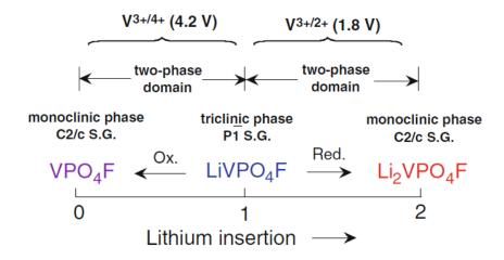
Figure 1-8. Schematic diagram of voltage-structure of  $Li_xVPO_4F$  ( $0 \le x \le 2$ ) material [62].
