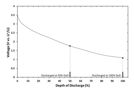
Figure 4-41. First discharge of oxidized MgMnSiO<sub>4</sub>/C treated in molten salts electrodes at C/10. The two discharged electrodes were stopped at 50% and 100% DoD (black crosses). 100% DoD was fixed to 174mAh. $g^{-1}$ .
