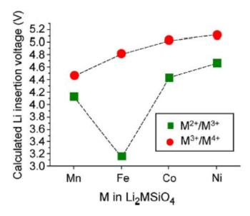
Figure 1-17. Computed lithium extraction voltage of  $M^{2+}/M^{3+}$  and  $M^{3+}/M^{4+}$  redox couple in Li<sub>2</sub>MSiO<sub>4</sub> (M=Mn, Fe, Co and Ni), adapted from [99].
