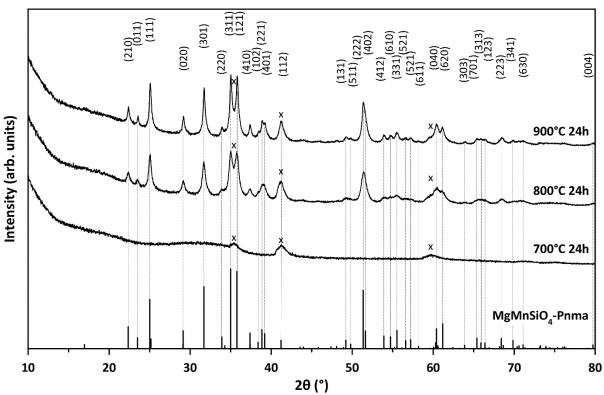
Figure 4-7. Powder X-Ray Diffraction patterns of MgMnSiO<sub>4</sub>/C pyrolyzed at 700°C for 24h, 800°C for 24h and 900°C for 24h, with heating and cooling rates of 5K.min<sup>-1</sup>. The main peaks of the MnO impurity are marked by a (x) symbol. The reflections of Pnma-MgMnSiO<sub>4</sub> are indicated by dotted vertical lines and their Miller indexes at the top of the figure.
