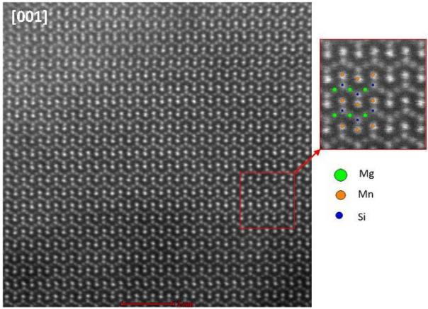
Figure 4-12. High-resolution STEM image of MgMnSiO $_4$ /C particle observed along the [001] orthorhombic zone axis. The general Mg, Mn and Si atomic positions are shown in inset, respectively in green, orange and blue.
