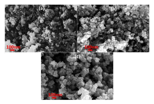
Figure 3-35. Scanning Electron Microscopy images of (a) LMS/C\_81 (Li<sub>2</sub>MnSiO<sub>4</sub>), (b) Li<sub>1.95</sub>Mn<sub>1.05</sub>Al<sub>0.05</sub>Si<sub>0.95</sub>O<sub>4</sub>/C and (c) Li<sub>1.90</sub>Mn<sub>1.10</sub>Al<sub>0.10</sub> Si<sub>0.90</sub>O<sub>4</sub>/C.
