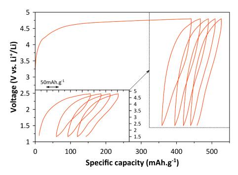
Figure 4-22. Galvanostatic cycling of MgMnSiO<sub>4</sub>/C treated in LiCl-KCl molten salts flux at 400°C for 40h at C/20 (1C=313mAh.g<sup>-1</sup>) and room temperature between 1.5V and 4.8V. The cycles 2 to 5 are shown in inset. The electrolyte and counter-electrode used are respectively based on LiPF<sub>6</sub> salt and a lithium counter-electrode.
