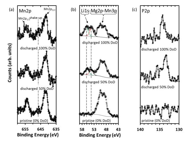
Figure 4-44. (a)Mn2p, (b) Li1s and (c) P2p XPS core spectra of oxidized MgMnSiO $_4$ /C treated in molten salts electrodes first discharged at C/10 at 0%, 50% and 100% DoD. Calibration with C1s at 284.8eV.
