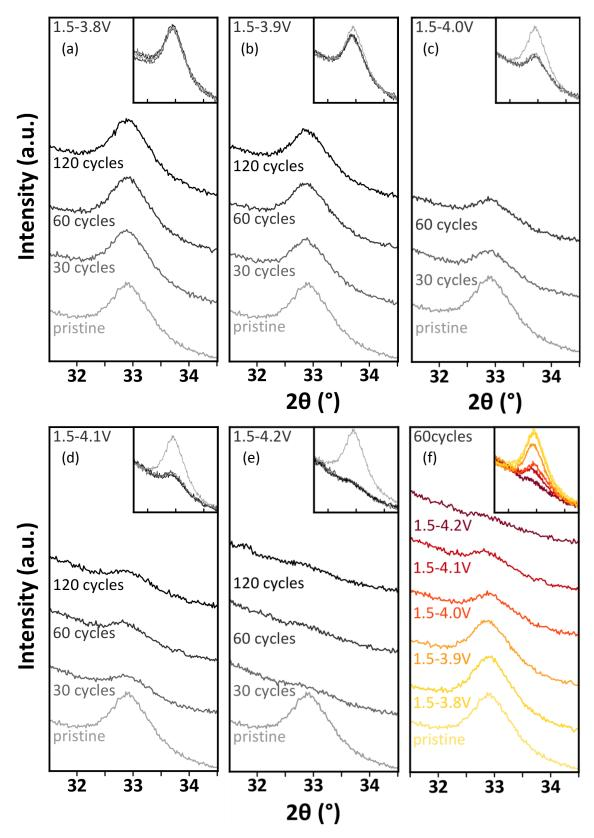
Figure 3-32. Ex-situ XRD patterns of discharged LMS/C\_81 electrodes after 30, 60 and 120 cycles for upper cut-off voltages of (a) 3.8V, (b) 3.9V, (c) 4.0V, (d) 4.1V, (e) 4.2V, (f) ex-situ XRD patterns of LMS/C\_81 electrodes after 120 cycles for all cut-off voltage conditions. The superimposed patterns are shown in insets in the same  $2\theta$  angle range.
