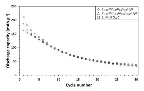
Figure 3-39. Cycling performance of  $Li_{2-x}Mn_{1+x}Al_xSi_{1-x}O_4/C$  (x=0, 0.05 and 0.1) electrodes at C/20 and room temperature between 1.5V and 4.8V. 1C=333 mA.g<sup>-1</sup>; 320 mA.g<sup>-1</sup> and 308mA.g<sup>-1</sup> respectively for x=0; 0.05 and 0.10.  $Li_{2-x}Mn_{1+x}Al_xSi_{1-x}O_4/C$ , with x=0, correspond to the LMS/C\_81 material.
