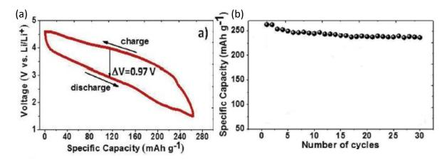
Figure 1-28. Second galvanostatic cycle of a  $Li_2MnSiO_4/C$  electrode between 1.5V and 4.8V at C/10 (a) and the associated reversible discharge capacity behavior as function of cycle number (b), adapted from [149].
