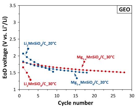
Figure 4-51. Evolution of End of Discharge voltage of  $Li_2MnSiO_4/C$  (squares) and  $Mg_{1-x}MnSiO_4/C$  (circles) based coin cells at 20°C (blue) and 30°C (red) as function of cycle number, for GEO cycling conditions.
