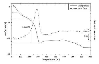
Figure 3-15. Evolution of the mass of a  $Li_2MnSiO_4/C$  material (straight line) and generated heat flow (dotted line) as a function of temperature, from RT to 900°C, under air, with heating rate of  $3K.min^{-1}$ .
