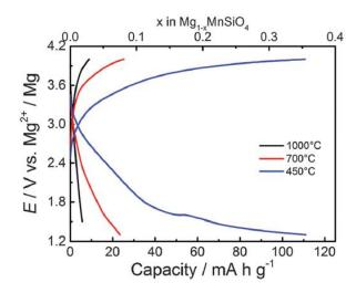
Figure 1-37. Galvanostatic first charge and first discharge of MgMnSiO₄ material synthesized at different temperatures, 1000°C (black), 700°C (red) and 450°C (blue), from [223].
