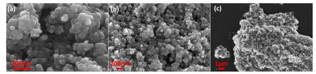
Figure 4-18. Scanning Electron Microscopy images of MgMnSiO $_4$ /C\_900 at different magnifications: (a) x300 000; (b) x100 000; (c) x20 000.
