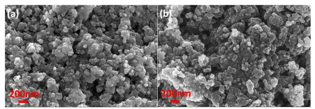
Figure 4-27. Scanning Electron Microscopy images of (a) MgMnSiO<sub>4</sub>/C and (b) oxidized MgMnSiO<sub>4</sub>/C treated in molten salts.
