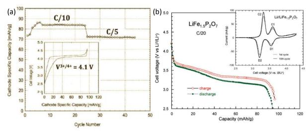
Figure 1-6. Reversible electrochemical capacity close to  $90\text{mAh.g}^{-1}$  depicted for carbothermally produced LiVP<sub>2</sub>O<sub>7</sub> positive electrode material using V<sup>3+/4+</sup> redox reaction at high voltage of 4.1V [55], (b) first charge-discharge profile for LiFe<sub>1.5</sub>P<sub>2</sub>O<sub>7</sub> at C/20, the inset shows the cyclic voltamogram recorded at a 0.1 mV.s<sup>-1</sup> sweep rate for the 1<sup>st</sup> and 10<sup>th</sup> charge-discharge cycle [56].
