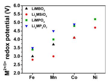
Figure 1-3. Potentials of  $M^{2+}/M^{3+}$  (M=Fe, Mn, Co and Ni) redox couples considering LiMBO<sub>3</sub>, Li<sub>2</sub>MSiO<sub>4</sub>, LiMPO<sub>4</sub> and Li<sub>2</sub>MP<sub>2</sub>O<sub>7</sub> materials, from [37].
