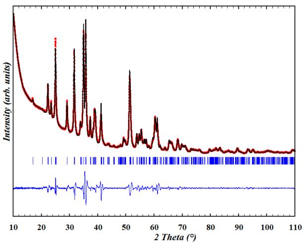
Figure 4-9. Full-pattern matching of MgMnSiO<sub>4</sub>/C from XRD data of MgMnSiO<sub>4</sub> collected with Cu anticathode (Cu  $K\alpha$ ), in the 10-110° 20 regions. An olivine lattice was used in the Pnma space group. Red markers: experimental data; black curve: refinement; blue tics: Bragg reflections; blue curve: least squares difference between experimental and refined data.
