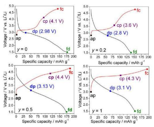
Figure 1-32. Firsts galvanostatic cycles of  $Li_2Fe_{1-y}Mn_ySiO_4/C$  (y=0, 0.2, 0.5, 1), from [138]. The indications on the curves correspond to ex-situ experiments that are not described here.
