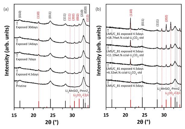
Figure 3-40. X-ray diffraction patterns of (a) pristine and exposed 4.5, 7, 14 and 30 days to air LMS/C\_81, (b) LMS/C\_81 exposed 4.5 days to air mixed with different weight fractions of commercial  $Li_2CO_3$  standard, ccial- $Li_2CO_3$ -std. All the reflections and Miller indexes of Pmn2<sub>1</sub>- $Li_2MnSiO_4$  and C2/c- $Li_2CO_3$  are indicated in (a), while only those used for quantitative analysis are displayed in (b).
