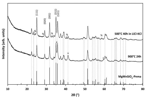
Figure 4-14. Powder X-Ray Diffraction patterns of MgMnSiO<sub>4</sub>/C pyrolyzed at 900°C for 24h alone and pyrolyzed in presence of LiCl-KCl molten salts flux at 500°C for 40h. The main peaks of MnO and Li<sub>2</sub>MnSiO<sub>4</sub> impurities are respectively marked by (x) and (%) symbols. The reflections of Pnma-MgMnSiO<sub>4</sub> are indicated by dotted vertical lines. The major reflections impacted by the antisite mixing are labelled by their Miller index on the top of the figure.
