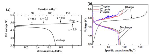
Figure 1-5. Galvanostatic charge-discharge cycles of (a) LiCoPO $_4$  at 0.1mA.cm $^{-2}$  and (b) LiNiPO $_4$ /C at C/10, respectively adapted from [48] and [49].
