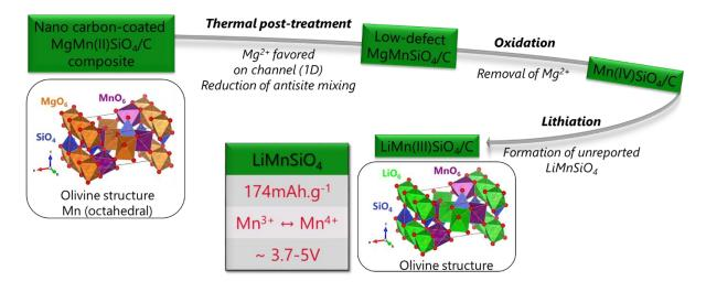
Figure 4-1. Scheme of the multi-step synthesis of LiMnSiO<sub>4</sub>/C from a MgMnSiO<sub>4</sub>/C precursor proposed in this chapter.
