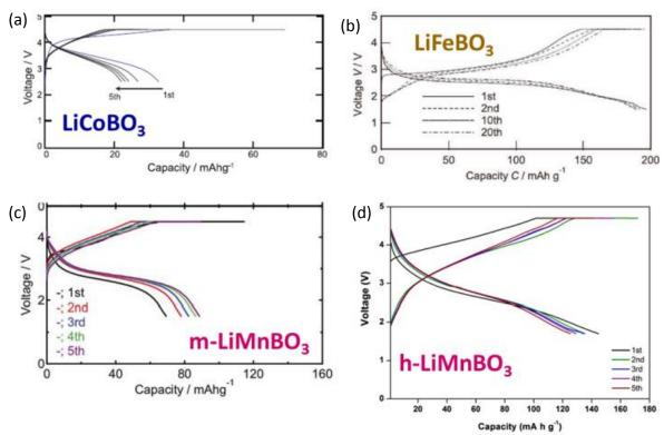
Figure 1-10. Galvanostatic charge-discharge curve of (a) LiCoBO<sub>3</sub> [75], (b) LiFeBO<sub>3</sub> [71], (c) monoclinic LiMnBO<sub>3</sub> [73], (d) hexagonal LiMnBO<sub>3</sub> [76] cycled at C/20, adapted from [77].
