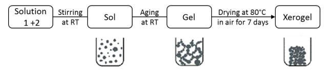
Figure 3-2. Scheme of the sol-gel process used for  $Li_2MnSiO_4$  and  $Li_2MnSiO_4/C$  materials synthesis. Illustrations are adapted from [239]. RT corresponds to room temperature.
