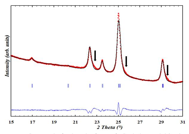
Figure 4-10. Full-pattern matching from the XRD data of MgMnSiO<sub>4</sub>/C collected with Cu anticathode (Cu  $K\alpha$ ), in the 15-30° 20 region. An olivine lattice was used in the Pnma space group. Red markers: experimental data; black curve: refinement; blue tics: Bragg reflections; blue curve: least squares difference between experimental and refined data; the black arrows indicate tails at the bottom of peaks that cannot be matched.
