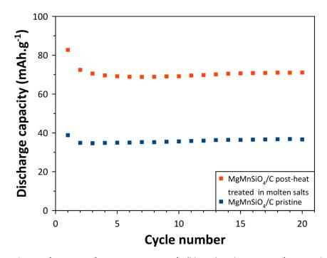
Figure 4-24. Cycling performance of pristine MgMnSiO<sub>4</sub>/C (blue  $\square$ ) and MgMnSiO<sub>4</sub>/C treated in molten salts (orange  $\square$ ) at C/20 (1C=313mAh.g<sup>-1</sup>) and room temperature between 1.5-4.8V. The electrolyte and counterelectrode used are respectively based on a LiPF<sub>6</sub> salt and a lithium counter-electrode.
