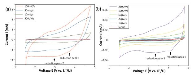
Figure 4-35. Cyclic voltammetry scans of oxidized MgMnSiO<sub>4</sub>/C at (a)  $500\mu V.s^{-1}$ - $100mV.s^{-1}$  sweep rates and (b)  $5\mu V.s^{-1}$ - $250\mu V.s^{-1}$  sweep rates between 1.5V and 4.8V at room temperature. Oxidation and reduction peaks are indicated by a number in order of appearance.
