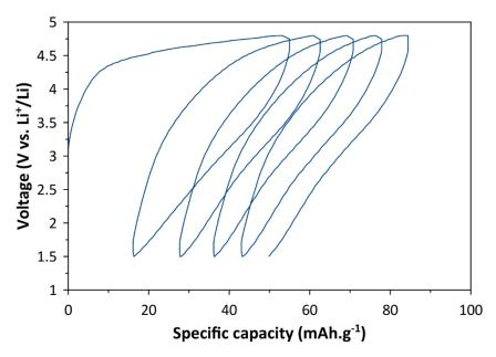
Figure 4-23. Galvanostatic cycling of MgMnSiO<sub>4</sub>/C at C/20 (1C=313mAh.g $^{-1}$ ) and room temperature between 1.5V and 4.8V. The electrolyte and counter-electrode used are respectively based on LiPF<sub>6</sub> salt and a lithium counter-electrode.
