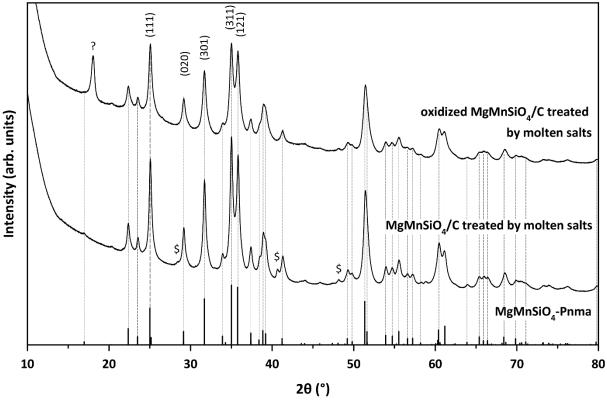
Figure 4-26. Powder X-Ray Diffraction patterns of pristine MgMnSiO<sub>4</sub>/C treated in molten salts and oxidized MgMnSiO<sub>4</sub>/C treated in molten salts. The KCl impurity peaks are labelled by a (\$) symbol. The additional peak appearing after the chemical oxidation is labelled with a (?) symbol.
