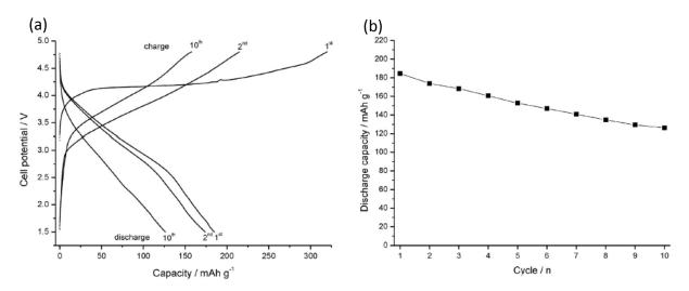
Figure 1-27. Galvanostatic cycles of a  $Li_2MnSiO_4/C$  material between 1.5V and 4.8V at C/50 and room temperature (a), and associated discharge capacity as a function of cycle number (b), adapted from [161].
