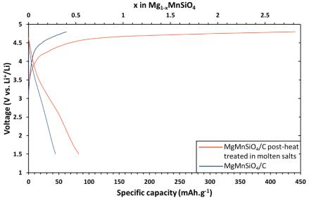
Figure 4-21. First galvanostatic charge and discharge of MgMnSiO<sub>4</sub>/C pyrolyzed at 900°C for 24h (blue line)) and MgMnSiO<sub>4</sub>/C treated in LiCl-KCl molten salts flux (orange line) electrodes between 1.5V and 4.8V at C/20 (1C=313mAh.g<sup>-1</sup>) and room temperature. The electrolyte and counter-electrode used are respectively based on a LiPF<sub>6</sub> salt and a lithium counter-electrode.
