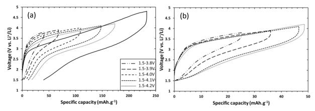
Figure 3-31. (a)  $2^{nd}$  and (b)  $120^{th}$  galvanostatic cycle of LMS/C\_81 respectively for the 3.8V, 3.9V, 4.0V, 4.1V and 4.2V upper cut-off voltages, at C/20 and room temperature.
