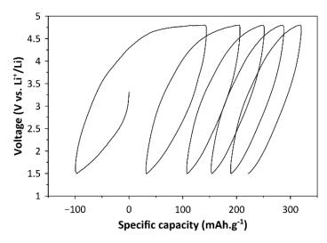
Figure 4-32. Galvanostatic cycling of oxidized MgMnSiO<sub>4</sub>/C at C/20 (1C=313mAh.g $^{-1}$ ) and room temperature between 1.5V and 4.8V.
