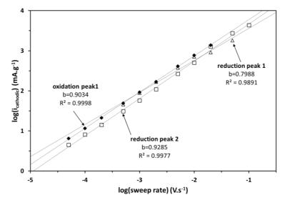
Figure 4-38. Evolution of reduction peaks current as a function of sweep rate for oxidized MgMnSiO $_4$ /C treated in molten salts. The reduction peaks here correspond to those of Figure 4-35. The slope, b, of Equation 4-4 is indicated as well as the correlation coefficient,  $R^2$ .
