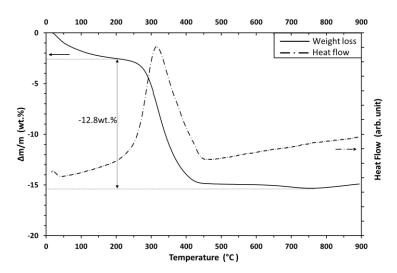
Figure 4-19. Evolution of the mass of MgMnSiO<sub>4</sub>/C pyrolyzed at 900°C for 24h (straight line) and generated heat flow (dotted line) as a function of temperature, from RT to 900°C, under air, with heating rate of  $3K.min^{-1}$ .
