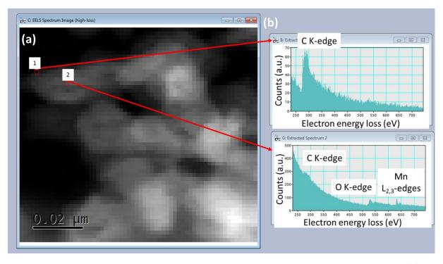
Figure 3-19. Scanning Transmission Electron Microscopy image in High-Angle Annular Dark-Field mode (a) and Electron Energy Loss Spectroscopy spectra in the 200-800eV range (b) of LMS/C\_81.
