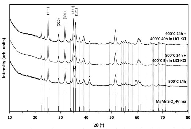
Figure 4-15. Powder X-Ray Diffraction patterns of MgMnSiO<sub>4</sub>/C pyrolyzed at 900°C for 24h and treated in LiCl-KCl molten salts flux at 400°C for 5h and 40h. The main peaks of MnO and Li<sub>2</sub>MnSiO<sub>4</sub> impurities are respectively marked by (x) and (%) symbols. The reflections of Pnma-MgMnSiO<sub>4</sub> are indicated by dotted vertical lines. The major reflections impacted by the antisite mixing are labelled by their Miller index on the top of the figure.
