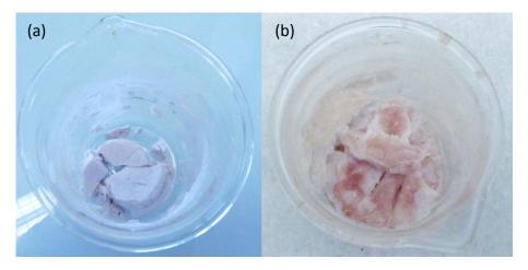
Figure 3-6. Pictures of the xerogels (a) from a sol without P123 polymer and (b) from a sol with intermediate P123 content.
