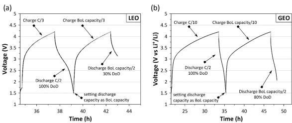
Figure 4-47. Examples of beginning of life capacity determination (1<sup>st</sup> galvanostatic cycle) and relevant C/rate and DoD conditions (2<sup>nd</sup> galvanostatic cycle for (a) LEO cycling and (b) GEO cycling) based on Li<sub>2</sub>MnSiO<sub>4</sub>/C cells at 20°C.
