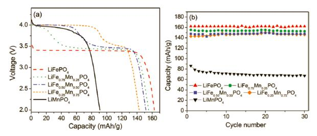
Figure 1-4. (a) Discharge profiles and (b) cycle-life of the LiFe<sub>1-x</sub> $Mn_xPO_4$  solid solution, x=0, 0.25, 0.50, 0.75 and 1, at C/20 [44].
