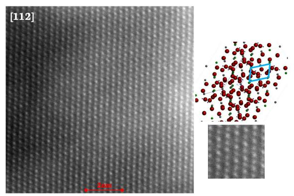
Figure 4-11. High-resolution STEM (HRSTEM) image of MgMnSiO<sub>4</sub>/C particle observed along the [112] orthorhombic zone axis of the olivine structure. The atomic positions of olivine structure are shown as a model along the [112] with  $O^{2-}$  in red,  $Mn^{2+}$  in green and  $Mg^{2+}$  in grey.
