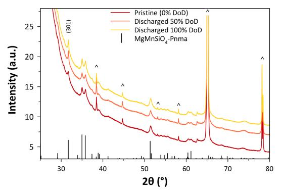
Figure 4-42. Ex-situ XRD patterns of oxidized MgMnSiO<sub>4</sub>/C treated in molten salts electrodes first discharged at C/10 at 0% (red), 50% (orange) and 100% DoD (yellow) (100% DoD=174mAh.g<sup>-1</sup>). The reflections of the aluminum current collector are indicated by (^) symbols. The Miller index of the Pnma-MgMnSiO<sub>4</sub> reflections that vary with DoD is indicated at the top of the figure.
