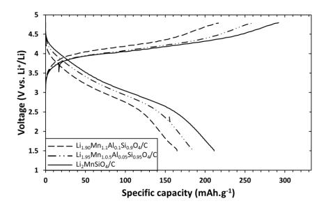
Figure 3-37. First galvanostatic cycle of  $Li_{2-x}Mn_{1+x}Al_xSi_{1-x}O_4/C$  (x=0, 0.05 and 0.1) electrodes at C/20 and room temperature between 1.5V and 4.8V. 1C=333 mA.g<sup>-1</sup>; 320 mA.g<sup>-1</sup> and 308mA.g<sup>-1</sup> respectively for x=0; 0.05 and 0.10.  $Li_{2-x}Mn_{1+x}Al_xSi_{1-x}O_4/C$ , with x=0, correspond to the reference material LMS/C\_81.
