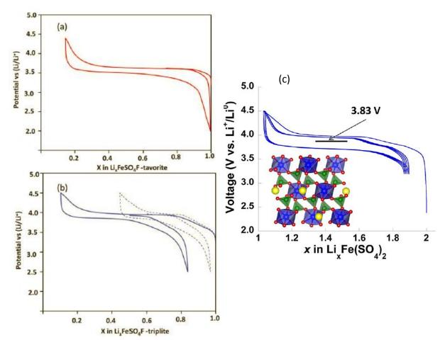
Figure 1-11. Galvanostatic charge-discharge of (a) tavorite LiFeSO<sub>4</sub>F, (b) triplite LiFeSO<sub>4</sub>F at C/10 [85] and (c)  $Li_2Fe(SO_4)_2$  [82].
