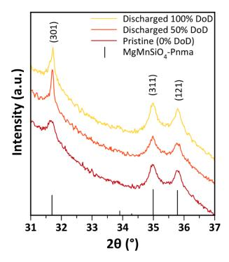
Figure 4-43. Zoom on the 31-37° 20 region of the ex-situ XRD patterns of oxidized MgMnSiO<sub>4</sub>/C treated in molten salts electrodes discharged at C/10 at 0% (red), 50% (orange) and 100% DoD (yellow) (10 % DoD=174mAh.g $^{-1}$ ). The reflections of the aluminum current collector are indicated by (^) symbols. The Miller indexes of the main Pnma-MgMnSiO<sub>4</sub> reflections are indicated at the top of the figure.
