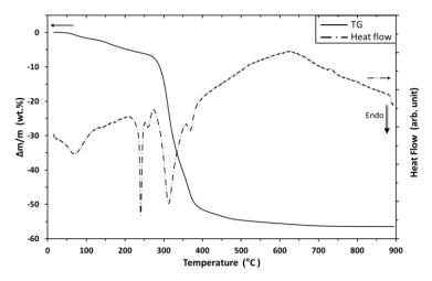
Figure 3-9. Evolution of the mass of the xerogel without P123 (straight line) and generated heat flow (dotted line) as a function of temperature, from RT to  $900^{\circ}$ C, under Ar, with heating rate of 5 K.min<sup>-1</sup>.
