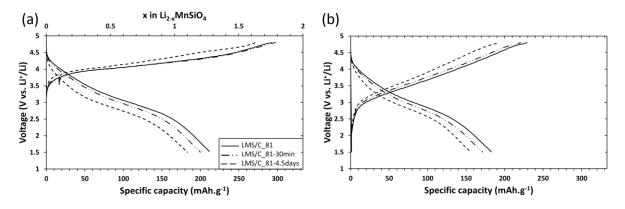
Figure 3-47. First (a) and second (b) galvanostatic cycle of pristine LMS/C\_81 (straight line), LMS/C\_81 exposed 30minutes to air, LMS/C\_81-30min (dotted-dashed line) and LMS/C\_81 exposed 4.5 days to air, LMS/C\_81-4.5 days (dashed line), at C/20 and room temperature between 1.5V and 4.8V.
