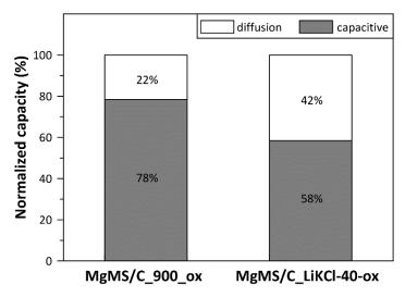
Figure 4-40. Histogram of normalized capacity contribution of diffusion, white area, and capacitance, shaded area, for oxidized MgMnSiO<sub>4</sub>/C and oxidized MgMnSiO<sub>4</sub>/C treated in molten salts.
