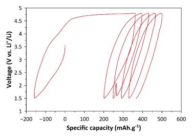
Figure 4-33. Galvanostatic cycling of oxidized MgMnSiO<sub>4</sub>/C treated in molten salts, at C/20 (1C=313mAh.g $^{-1}$ ) and room temperature between 1.5V and 4.8V.
