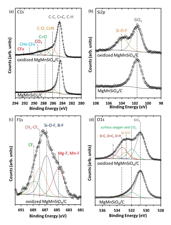
Figure 4-29. XPS core C1s (a), Si2p (b), F1s (c) and O1s (d) normalized spectra of MgMnSiO<sub>4</sub>/C and oxidized MgMnSiO<sub>4</sub>/C. Calibration with Si2p component of SiO<sub>4</sub> at 101.7eV.
