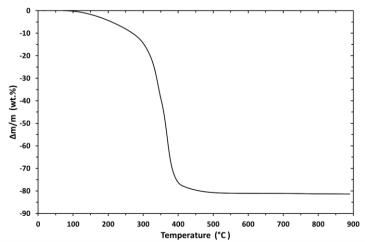
Figure 4-4. Evolution of the mass of the Mg,Mn,Si xerogel with intermediate content of P123 (straight line) as a function of temperature, from RT to 900°C, under Ar, with heating rate of 5 K.min<sup>-1</sup>.
