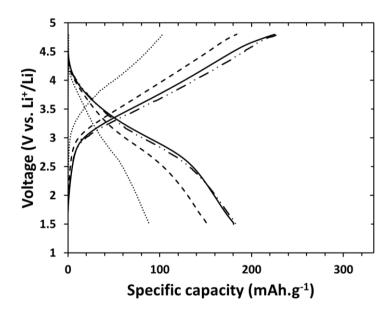
Figure 3-22. Second galvanostatic cycles of LMS, LMS/C\_57, LMS/C\_81 and LMS/C\_169 electrodes at C/20 and room temperature between 1.5V and 4.8V. Dotted line, dashed line, dotter-dashed mixed line and straight line correspond to LMS, LMS/C\_57, LMS/C\_81 and LMS/C\_169 materials respectively.
