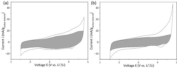
Figure 4-39. Cyclic voltammetry scan at  $50\mu V.s^{-1}$  of (a) oxidized MgMnSiO<sub>4</sub>/C and (b) oxidized MgMnSiO<sub>4</sub>/C treated in molten salts, between 1.5V and 4.8V at room temperature. The representation is inspired from [297].
