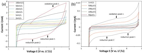
Figure 4-37. Cyclic voltammetry scans of oxidized MgMnSiO<sub>4</sub>/C treated in molten salts at (a)  $2mV.s^{-1}$ - $100mV.s^{-1}$  sweep rates and  $50\mu V.s^{-1}$ - $1mV.s^{-1}$  sweep rates between 1.5V and 4.8V at room temperature. Oxidation and reduction peaks are indicated by a number in order of appearance.
