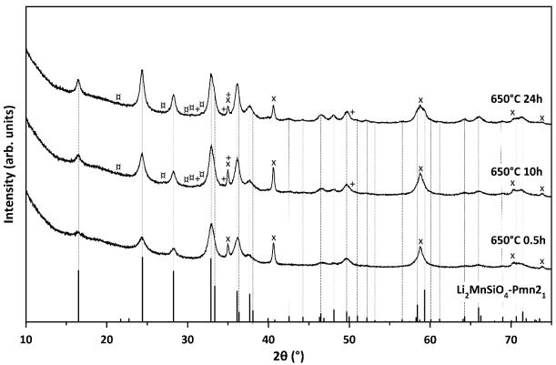
Figure 3-14. Powder X-Ray Diffraction patterns of  $\text{Li}_2\text{MnSiO}_4/\text{C}$  described in the Pmn2<sub>1</sub> space group and pyrolyzed at 650°C in argon for 0.5h, 10h and 24h. The main peaks of each impurity are displayed and denoted as the following:  $\text{Li}_2\text{CO}_3$  (x),  $\text{Li}_2\text{SiO}_3$  (\*),  $\text{Mn}_2\text{SiO}_4$  (+) and MnO (x). The reflections of Pmn2<sub>1</sub>-Li<sub>2</sub>MnSiO<sub>4</sub> are indicated by dotted vertical lines.
