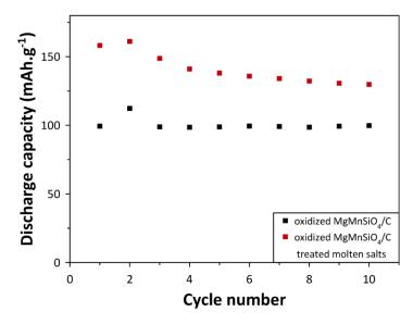
Figure 4-34. Cycling performance of oxidized MgMnSiO<sub>4</sub>/C (black  $\square$ ) and oxidized MgMnSiO<sub>4</sub>/C treated in molten salts (red  $\square$ ) at C/20 (1C=313mAh.g<sup>-1</sup>) and room temperature between 1.5-4.8V.
