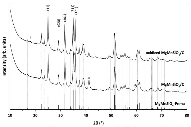
Figure 4-25. Powder X-Ray Diffraction patterns of pristine MgMnSiO $_4$ /C and oxidized MgMnSiO $_4$ /C. The additional peak appearing after the chemical oxidation is labelled with a (?) symbol.
