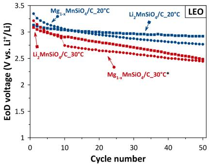
Figure 4-50. Evolution of End of Discharge voltage of Li<sub>2</sub>MnSiO<sub>4</sub>/C (squares) and Mg<sub>1-x</sub>MnSiO<sub>4</sub>/C (circles) based coin cells at 20°C (blue) and 30°C (red) as function of cycle number, for LEO cycling conditions. (\*) The cell containing Mg<sub>1-x</sub>MnSiO<sub>4</sub>/C and cycled at 30°C (blue circles) was charged at C/10 instead of C/3 for the 9 first cycles and then charged at C/3.
