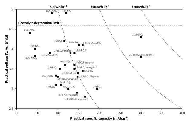
Figure 1-12. Practical voltage (V vs.  $Li^+/Li$ ) of polyanionic materials as a function of practical specific capacity (mAh.g<sup>-1</sup>) inspired from [88], the isovalue lines represent the energy density of the positive electrode (Wh.kg<sup>-1</sup>).
