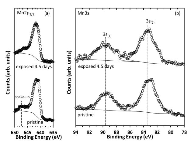
Figure 3-44. XPS Mn2 $p_{3/2}$  (a) and Mn3s (b) spectra of pristine and exposed 4.5 days to air LMS/C\_81 materials. Split peaks of Mn3s at high and low binding energies are respectively denoted  $3s_{(1)}$  and  $3s_{(2)}$ . Spectra were calibrated with the "SiO<sub>4</sub>" O1s component at 530.5eV.
