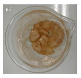
Figure 4-3. Pictures of (a) a gel and (b) a xerogel, both containing Mg, Mn and Si precursors together with P123 as a carbon source.
