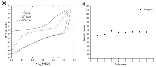
Figure 1-20. (a) First galvanostatic cycles of  $\text{Li}_2\text{FeSiO}_4/\text{C}$  at C/30 [95] and (b) cycling performance of  $\text{Li}_2\text{FeSiO}_4/\text{C}$  at C/16 and 60°C [94].
