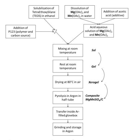
Figure 4-2. Protocol used for the sol-gel synthesis of MgMnSiO<sub>4</sub>/C materials in inert atmosphere.
