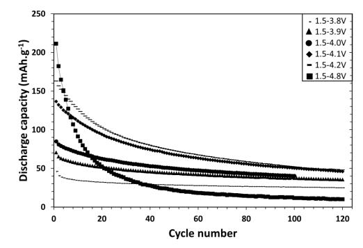
Figure 3-30. Cycling performance of LMS/C\_81 over 120 cycles for different upper cut-off voltages, 3.8V (small dash), 3.9V (triangle), 4.0V (circle), 4.1V (diamond), 4.2V (big dash) and 4.8V (square).
