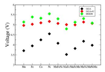
Figure 1-35. Voltage prediction of LiMSiO<sub>4</sub> (M=Mn, Fe, Co, Ni) (V vs.  $Li^+/Li$ ) according to several computation methods [225].
