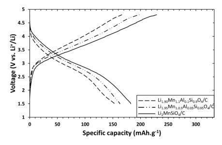
Figure 3-38. Second galvanostatic cycle of  $Li_{2-x}Mn_{1+x}Al_xSi_{1-x}O_4/C$  (x=0, 0.05 and 0.1) electrodes at C/20 and room temperature between 1.5V and 4.8V. 1C=333 mA.g<sup>-1</sup>; 320 mA.g<sup>-1</sup> and 308mA.g<sup>-1</sup> respectively for x=0; 0.05 and 0.10.  $Li_{2-x}Mn_{1+x}Al_xSi_{1-x}O_4/C$ , with x=0, correspond to the reference material LMS/C 81.
