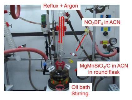
Figure 4-6. Picture of the chemical oxidation set-up including: a round flask containing a dispersion of  $MgMnSiO_4/C$  in acetonitrile heated by an oil bath at  $60^{\circ}C$  and stirred continuously; a water-cooled condenser which condenses ACN vapors and an isobar dropping funnel containing a solution of  $NO_2BF_4$  in ACN.
