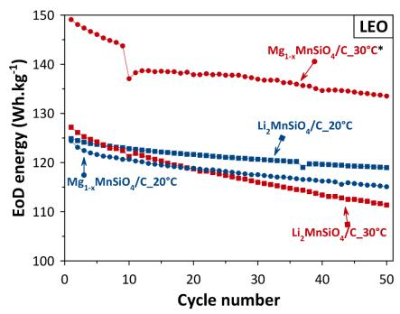
Figure 4-48. Evolution of End of Discharge energy of Li<sub>2</sub>MnSiO<sub>4</sub>/C (squares) and Mg<sub>1-x</sub>MnSiO<sub>4</sub>/C (circles) coin cells at 20°C (blue) and 30°C (red) as function of cycle number, for LEO cycling conditions. (\*) The cell containing material B and cycled at 30°C (blue circles) was charged at C/10 instead of C/3 for the 9 first cycles and then charged at C/3.
