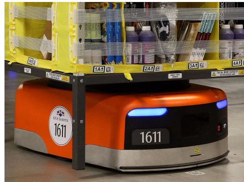
Figure 1.12: Kiva robot of amazon
