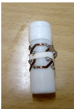
Figure 1.13. A saddle coil designed for rapid dissolution. A sample holder can be inserted from the top of the VTI into the active volume of the coil.
