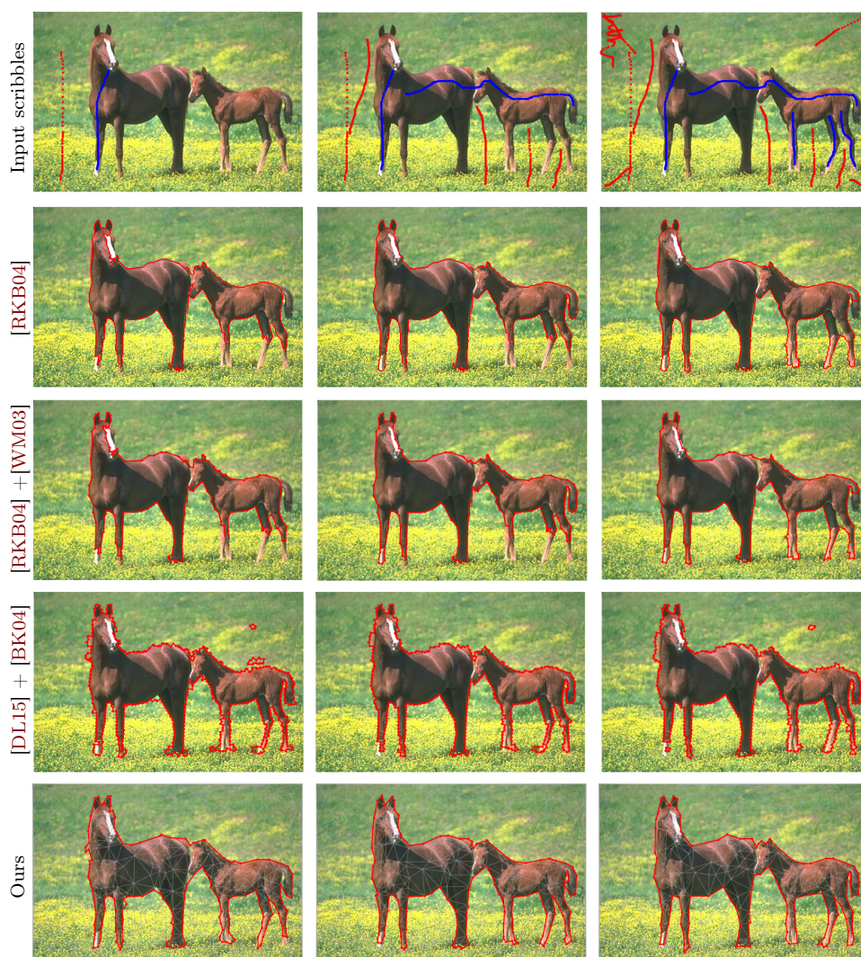
Figure 6.16: Comparisons with two-steps object contouring methods given different sets of input scribbles. The GrabCut pixel-based segmentation [RKB04] requires many input scribbles to correctly capture horse silhouettes (see the bottom parts of the legs). Converting the output pixel chains to polygons using Douglas-Peucker algorithm [WM03] accentuates their defects, whereas pre-segmenting the input image into polygonal superpixels [DL15] only give satisfactory results when small superpixels are used, i.e. for high output complexity. In contrast, our Delaunay point process produces low complexity polygons that accurately capture the horses, even when only two scribbles are provided.
