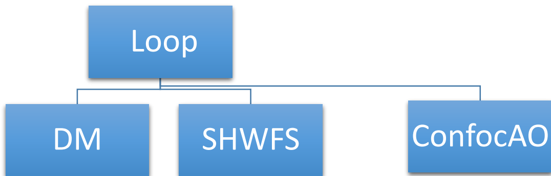
Figure 2.11 – Closed loop class diagram. The closed loop class interacts mainly with the DM and SHWFS, and occasionally with the microscope class to open the laser shutter for example.
