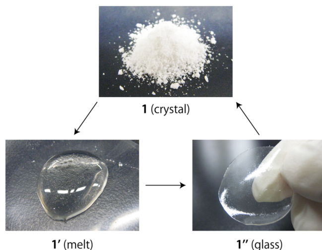
Figure 1.5: Photographs of 1 , the crystal, 1' , the melt and 1'' the glass. Figure taken from [195].
