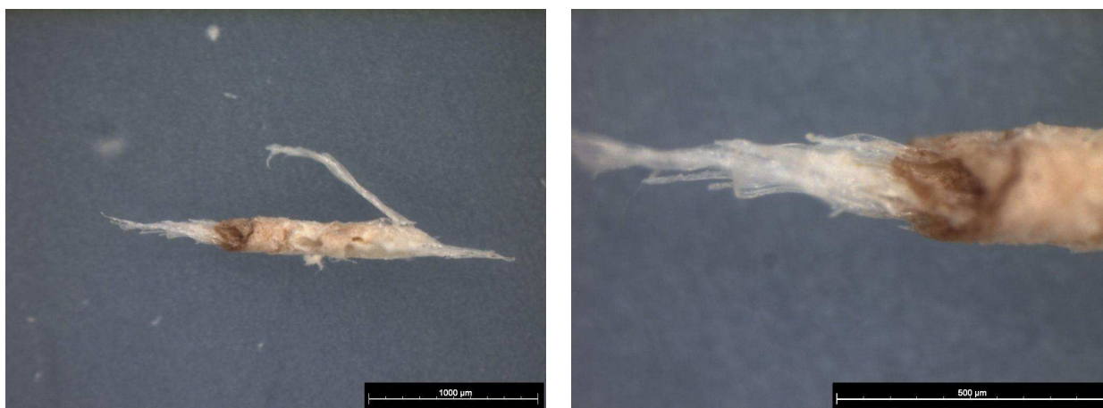
Figure 146: TMP shives blocked the screen apertures
