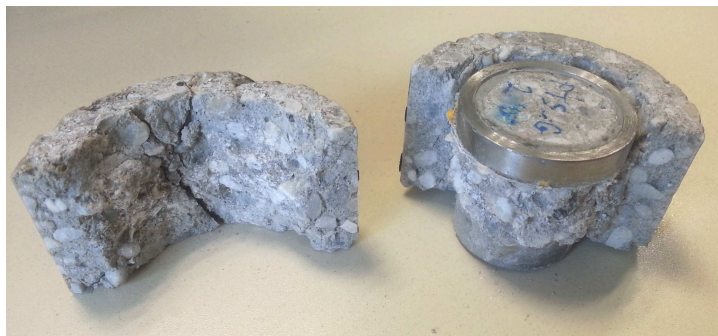
FIGURE 2.29: View from the inside of a concrete specimen subjected to a confining pressure of 100 MPa
