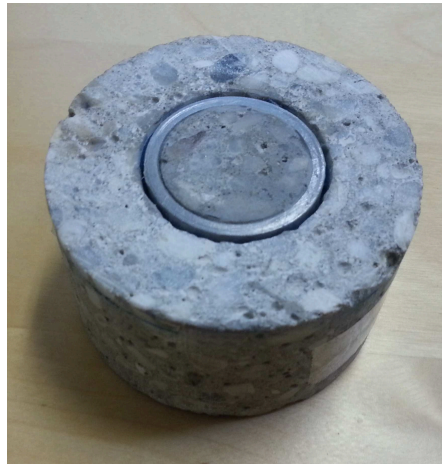
FIGURE 2.19: Concrete sample equipped with a ring
