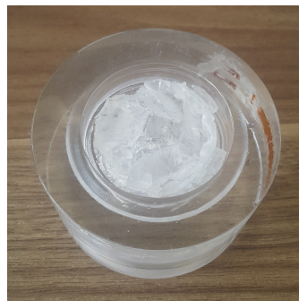
FIGURE 2.23: PMMA specimen with a ligament length of 20mm, central part damaged under compression
