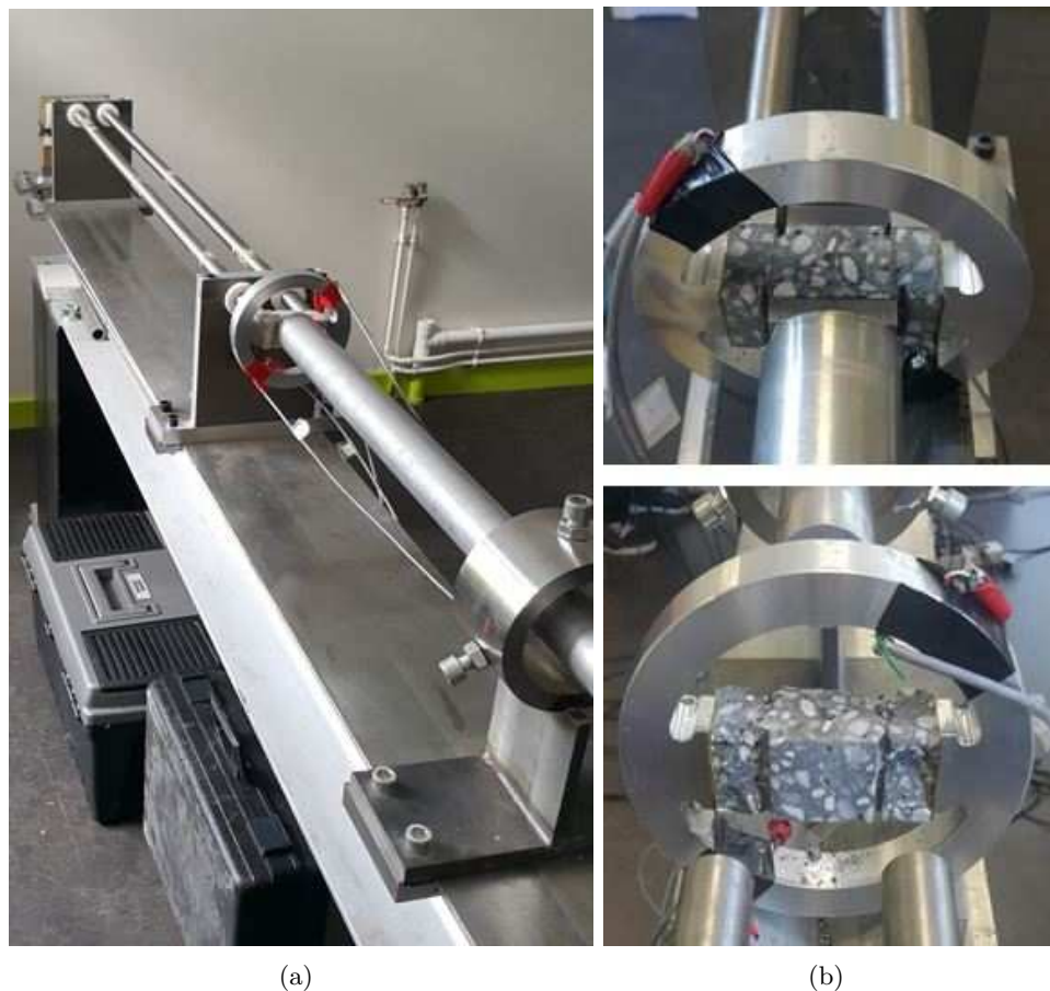
FIGURE 3.42: Experimental device used for dynamic shear tests (a) General view of the setup (b) zoom on a concrete sample with the confinement ring before and after testing
