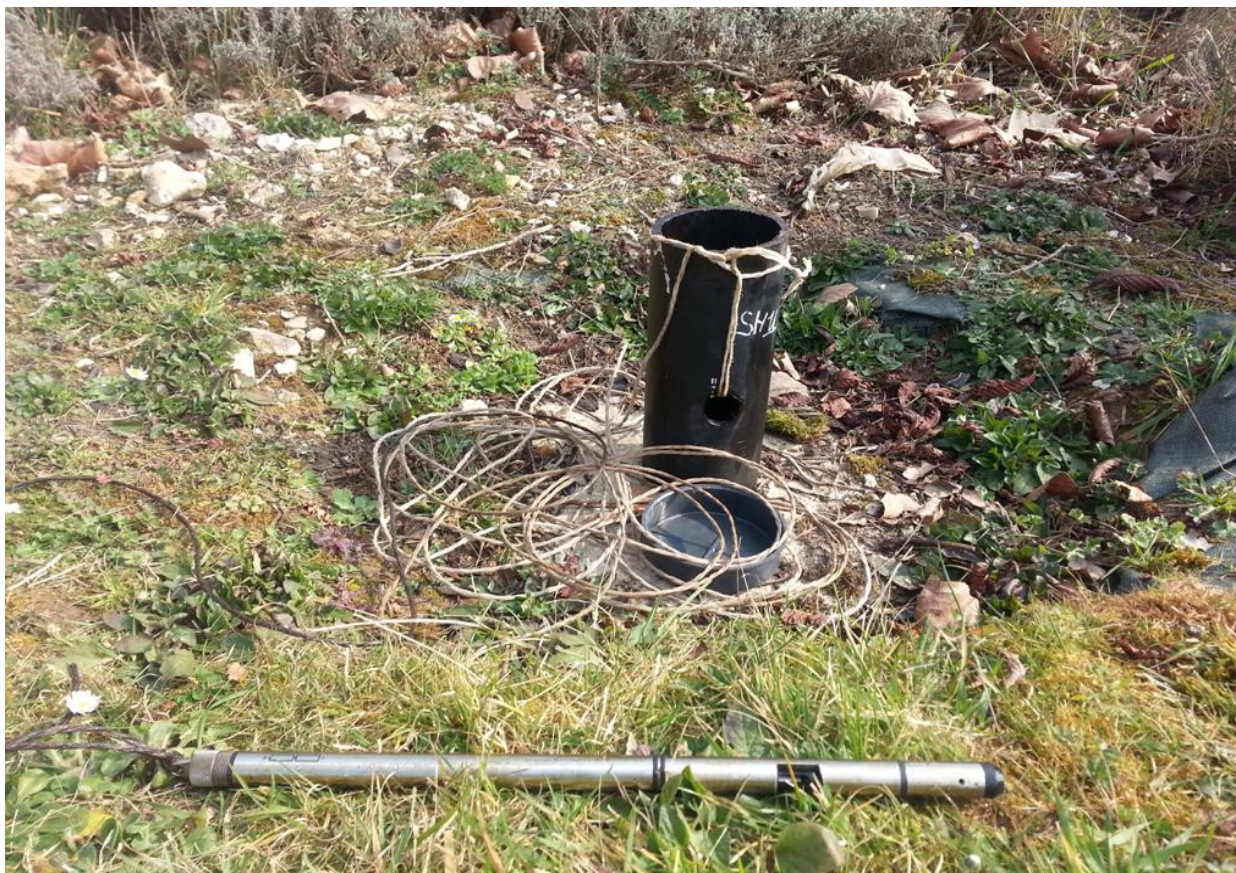
Figure 2.9: The INW smart sensor which was used to measure geochemical parameters such as the concentration of total dissolved solids and groundwater electrical conductivity.
