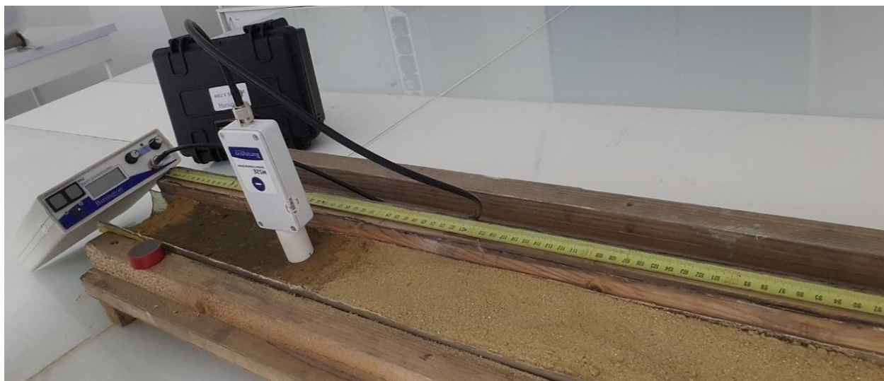
Figure 3.17: The MS2 Bartington equipment used to conduct the magnetic susceptibility measurements on a soil core.
