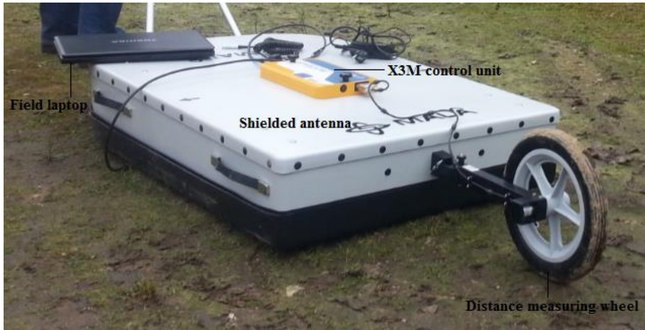
Figure 3.14: The Mala Geoscience GPR system used to acquire the GPR data. The system contains a shielded antenna, a control unit (X3M), a distance measuring wheel and a field laptop.
