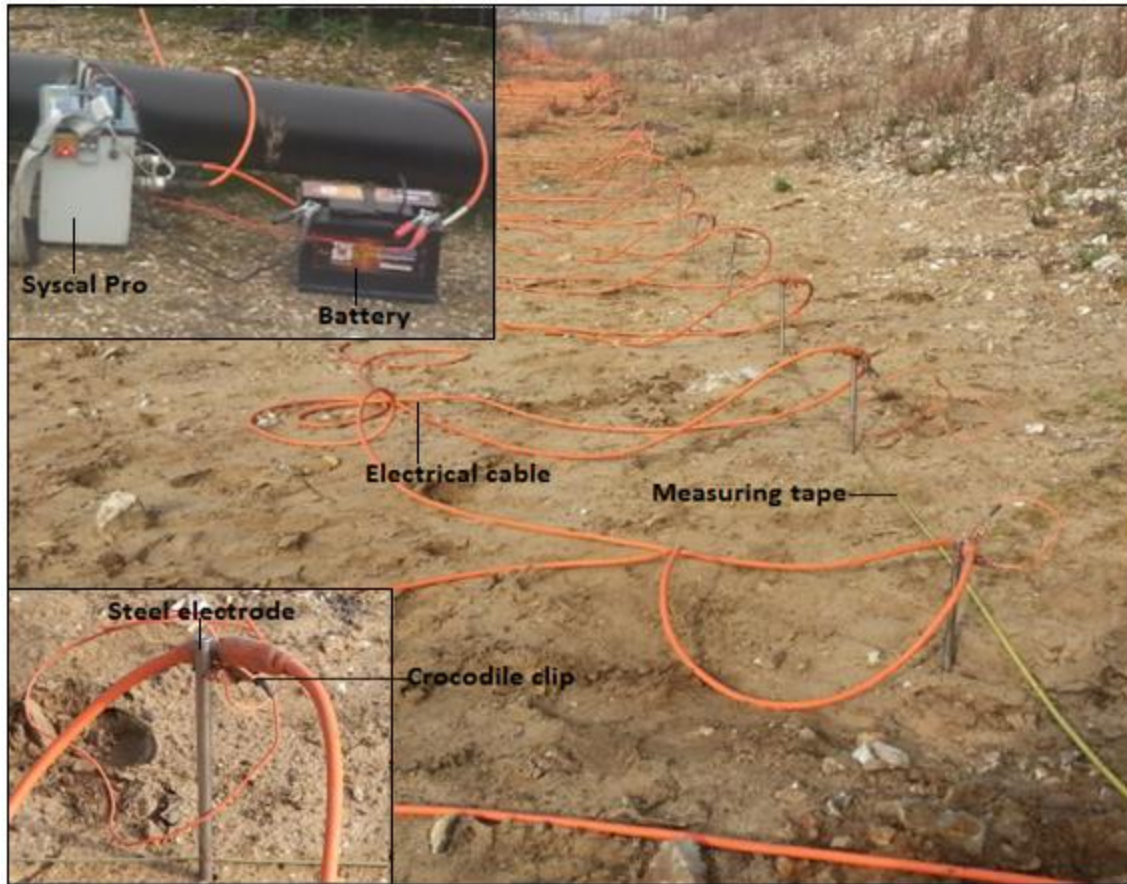
Figure 3.10: The field setup and the equipment used in the electrical resistivity tomography survey.
