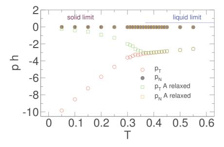
Figure 2.3: Integrals of the tangential and normal pressure profiles as a function of temperature T. Using Equation (2.23) gives the surface tension  $\gamma \approx 1.5$  close to the liquid-glass transition.
