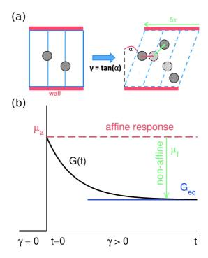
Figure 2.4: Panel (a): The scheme of the simple shear experiment with  $\gamma$  being the shear strain, red arrow the affine displacement and green arrow additional non-affine displacement. Panel (b): Sketch of the Eq. (2.25) and Eq. (2.26) with G(t) being the shear relaxation modulus (black solid line),  $G_{eq}$  the equilibrium shear modulus (blue solid horizontal line),  $\mu_a$  the affine shear elasticity (red dashed horizontal line),  $\mu_f$  the non-affine shear elasticity.
