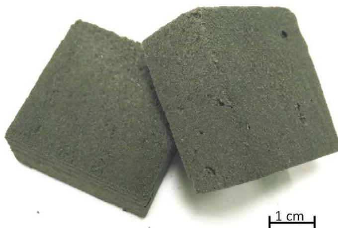
Fig. IV-1. Example of tannin-furanic foam samples prepared and tested in this work.
