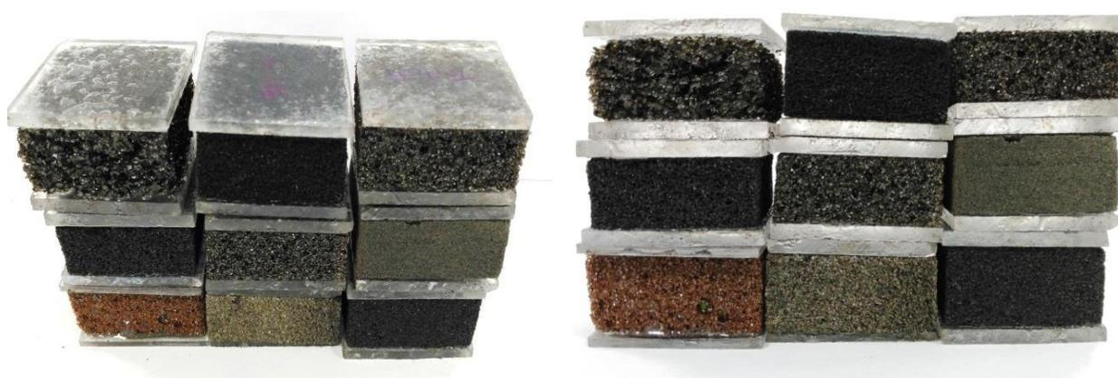
Fig. VI-1. Tannin-based foams glued to plastic plates, ready for compression test.
