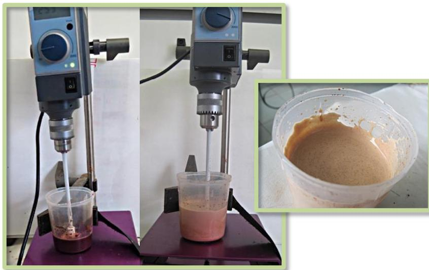
Fig. II-1. Preparation of a liquid meringue tannin-based foam.
