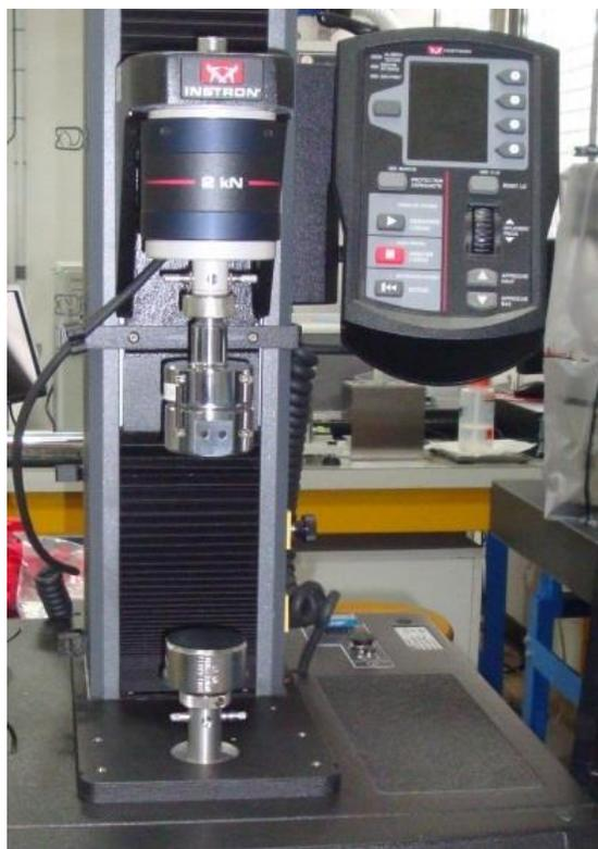
Fig. IV-3. Universal test machine INSTRON 5944 equipped with its compression plates.
